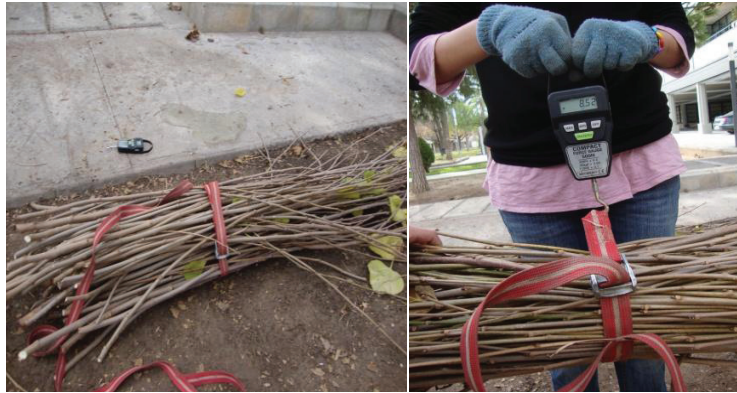
Figure 1. From left to right: bundles of pruned branches; weighting process with a dynamometer
