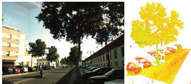
Figure 15. From left to right: picture of scanned trees in the urban area; obtained scan data, where elements different to the tree must be filtered
