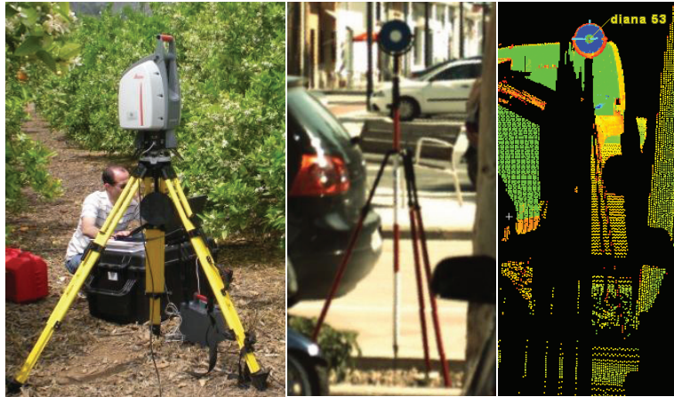
Figure 13. From left to right: Leica ScanStation 2 equipment with necessary accessories; tripod-mounted HDS target; scanned target
