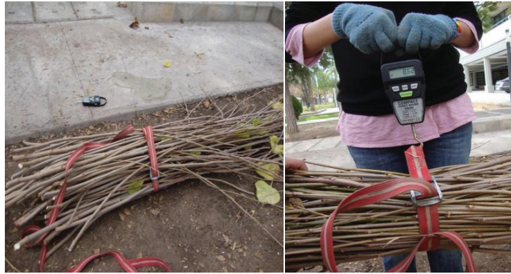
Figure 1. From left to right: bundles of pruned branches; weighting process with a dynamometer
