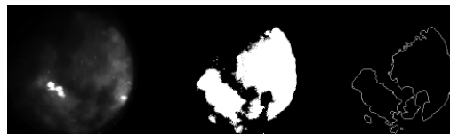
Fig. 4 – Scheme of processing steps. From left to right: original image, binary image of the flame area and binary image of the flame contour
