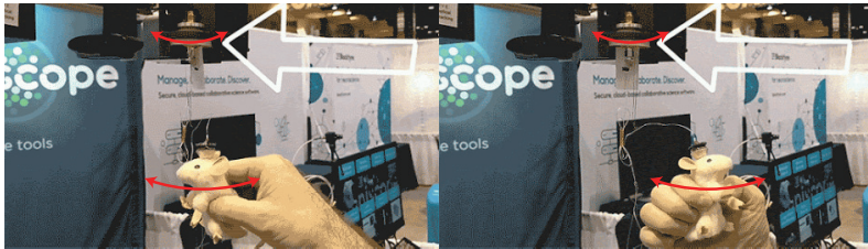
Figure 4.16: Commutator actively following headstage orientation.
