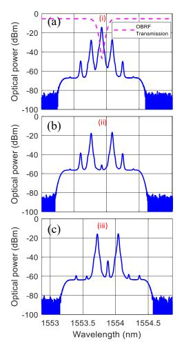
Figure 2. Optical spectra of: (a) Quadrature bias modulated signal (System A) before OBRF, (b) Quadrature bias modulated signal (System A) after OBRF, and (c) Carrier suppressed modulated signal (System B).
