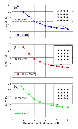
Figure 5. EVM performance of the System B transmitting a 16-QAM data signal with 500 MHz bandwidth for: (a) OB2B, (b) 10 km SSMF, and (c) full hybrid link with 10 km SSMF and 1.5 m long FSO channel . Insets show the constellations.
