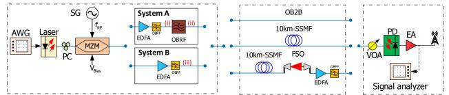
Figure 1. Experimental setup of a DML data signal modulation, carrier supression and RoF and RoFSO transmission. AWG: arbitrary waveform generator, PC: polarization controller, MZM: Mach-Zehnder modulator, SG: RF signal generator, EDFA: erbium doped fiber amplifier, OBPF: optical bandpass filter, OBRF: optical band-rejection filter, OB2B: optical back-to-back, SSMF: standard single mode fiber, FSO: free space optics, VOA: variable attenuator, EA: electrical amplifier, PD: photodetector.
