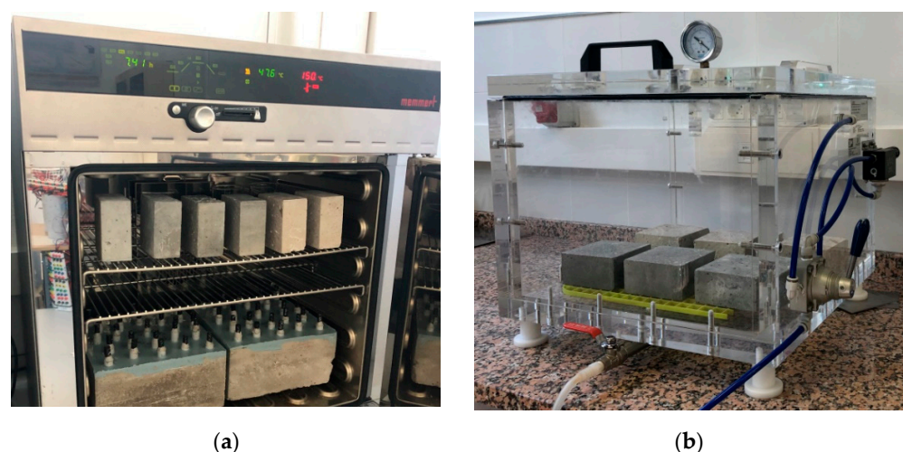
Figure 2. Water absorption set up: (a) specimens in the oven; (b) specimens in the vacuum chamber.
