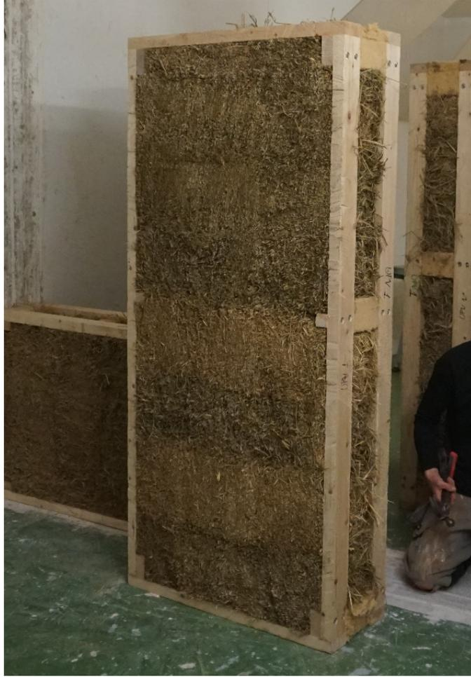
**Figure 3.4.** Straw panel in the transmission chamber
