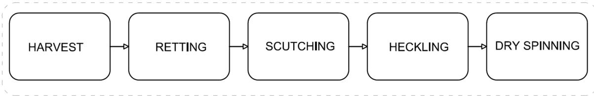
**Figure 1.2.** Flax, jute, and hemp manufacturing process
