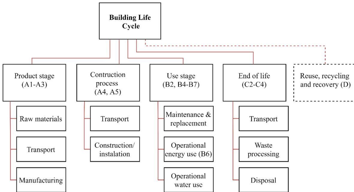
**Figure 4.2.** Building life cycle (with modules A1-D) according to EN15804 (2020), Module D and module B3 (repair) are outside the scope of the study.
