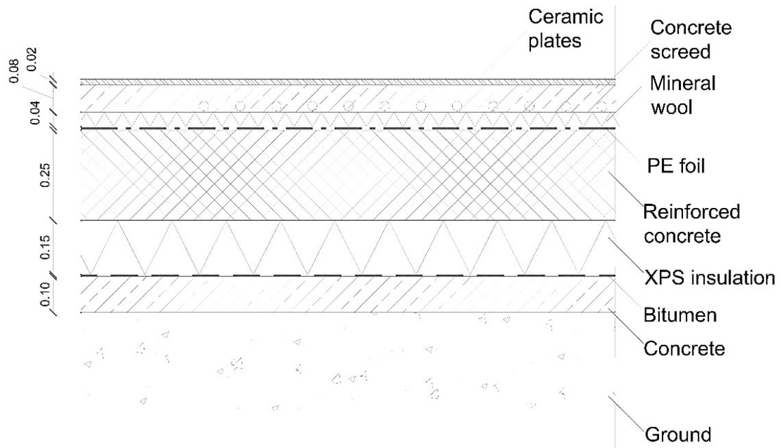
**Figure D11.** Section of the ground floor
