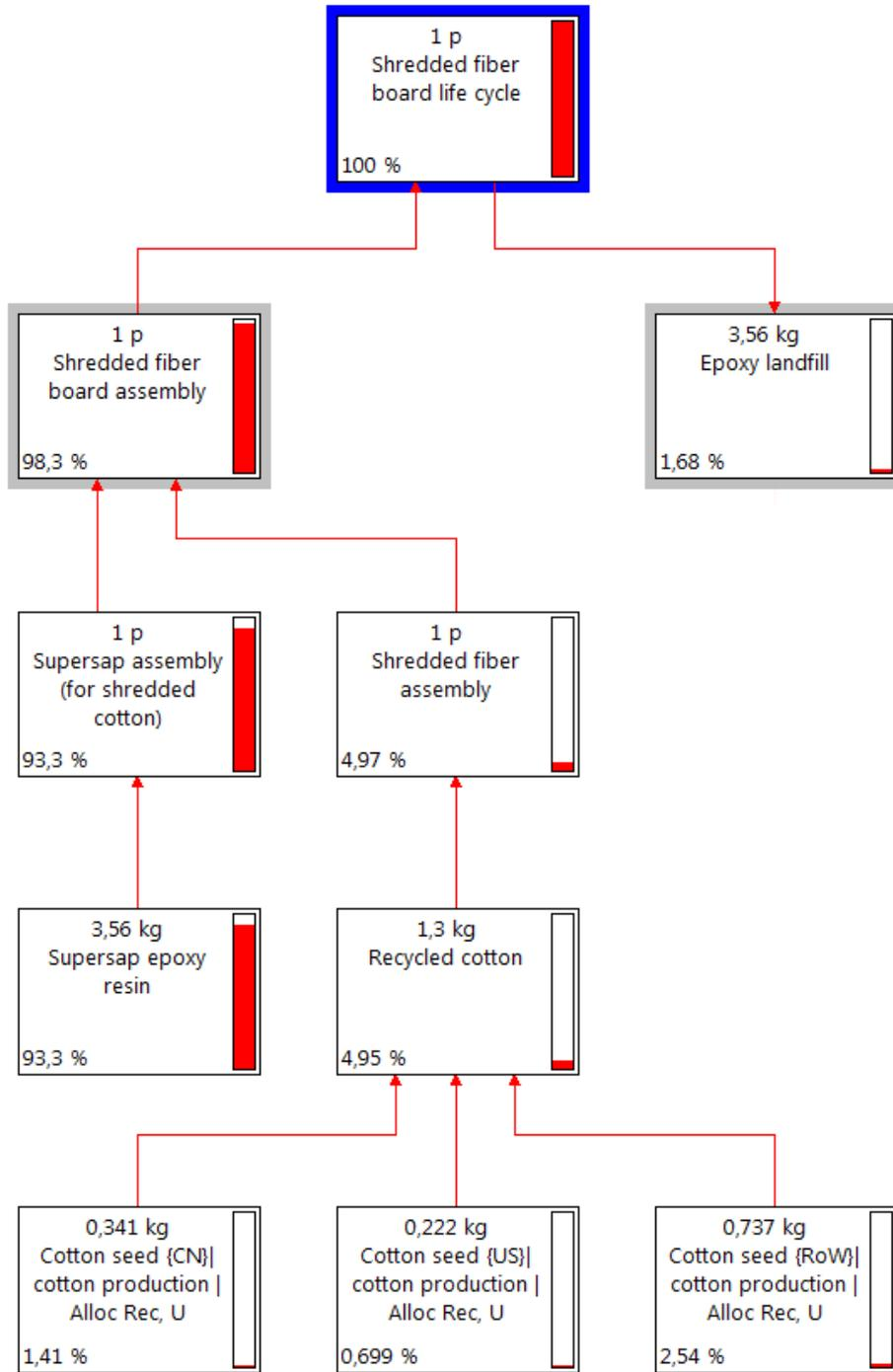
**Figure 1.11.** Network of the life cycle of the shredded cotton composite board
