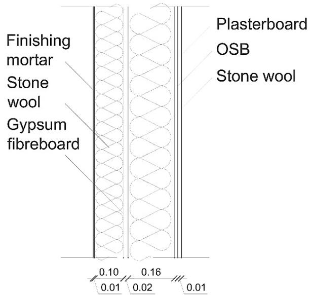
**Figure D9.** Section of the exterior walls (W1)
