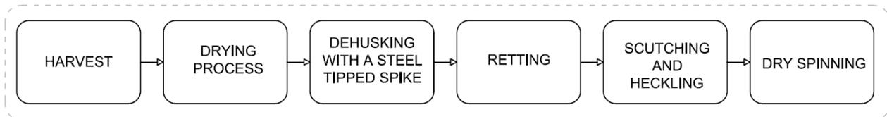
**Figure 1.3.** Coir manufacturing process
