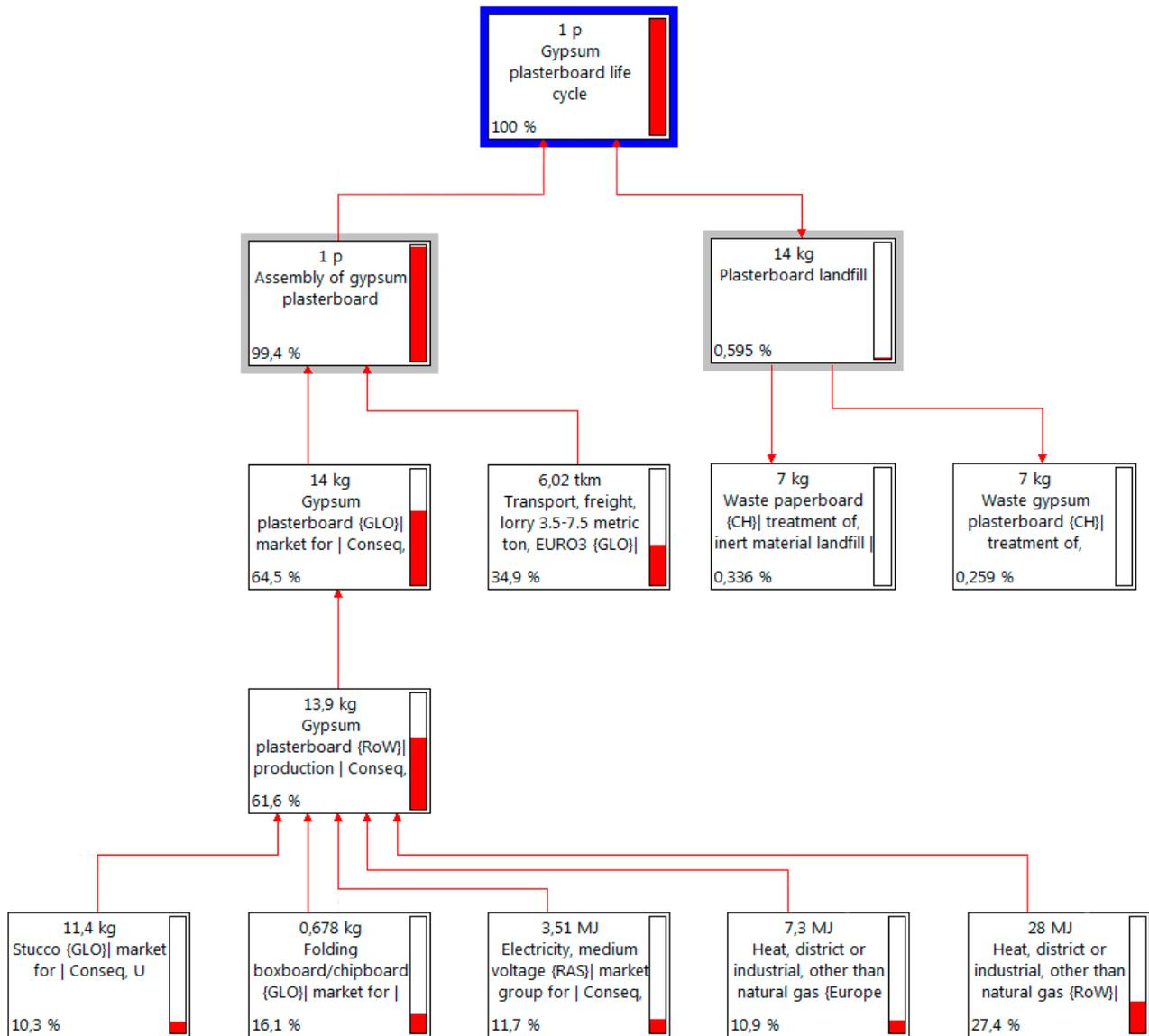
**Figure 1.6.** Network of the life cycle of gypsum plasterboard
