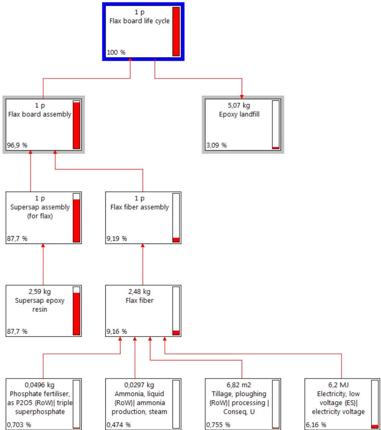
**Figure 1.8.** Network of the life cycle of the flax composite board
