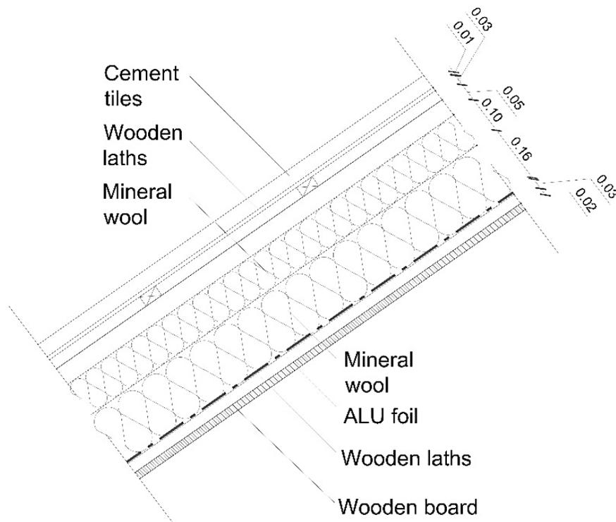
**Figure D12.** Section of the roof (R1)
