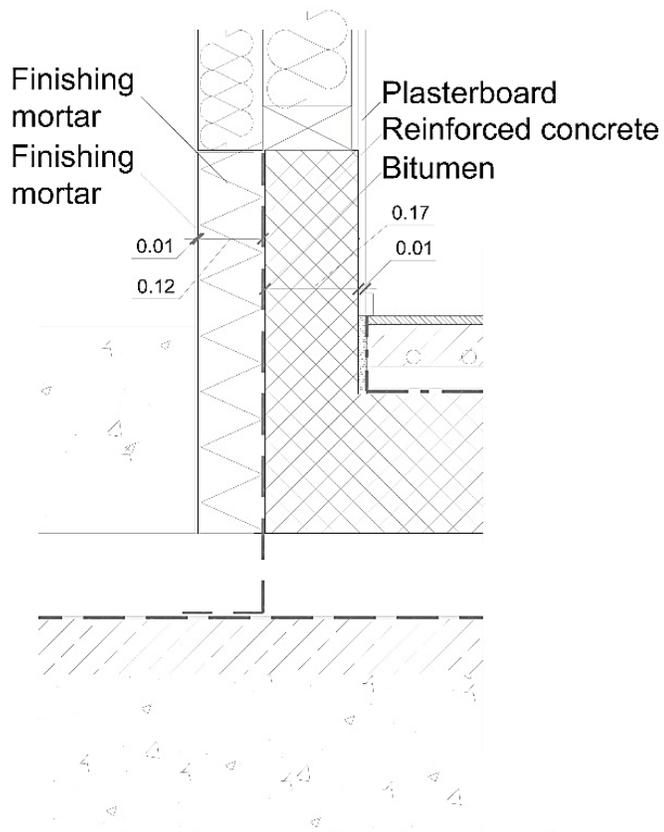
**Figure D10.** Section of the exterior wall ground floor bottom (W2)
