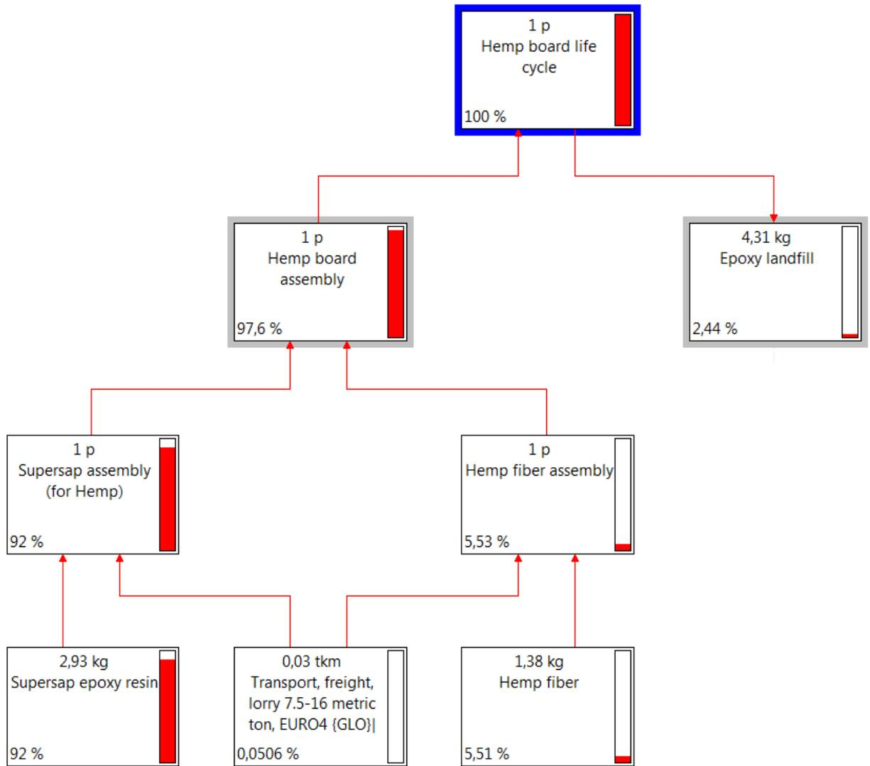
**Figure 1.10.** Network of the life cycle of the hemp composite board
