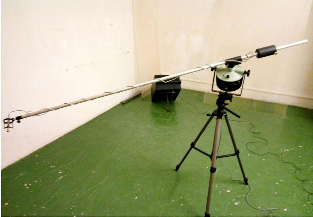
**Figure A7.** Rotating microphone and sound source
