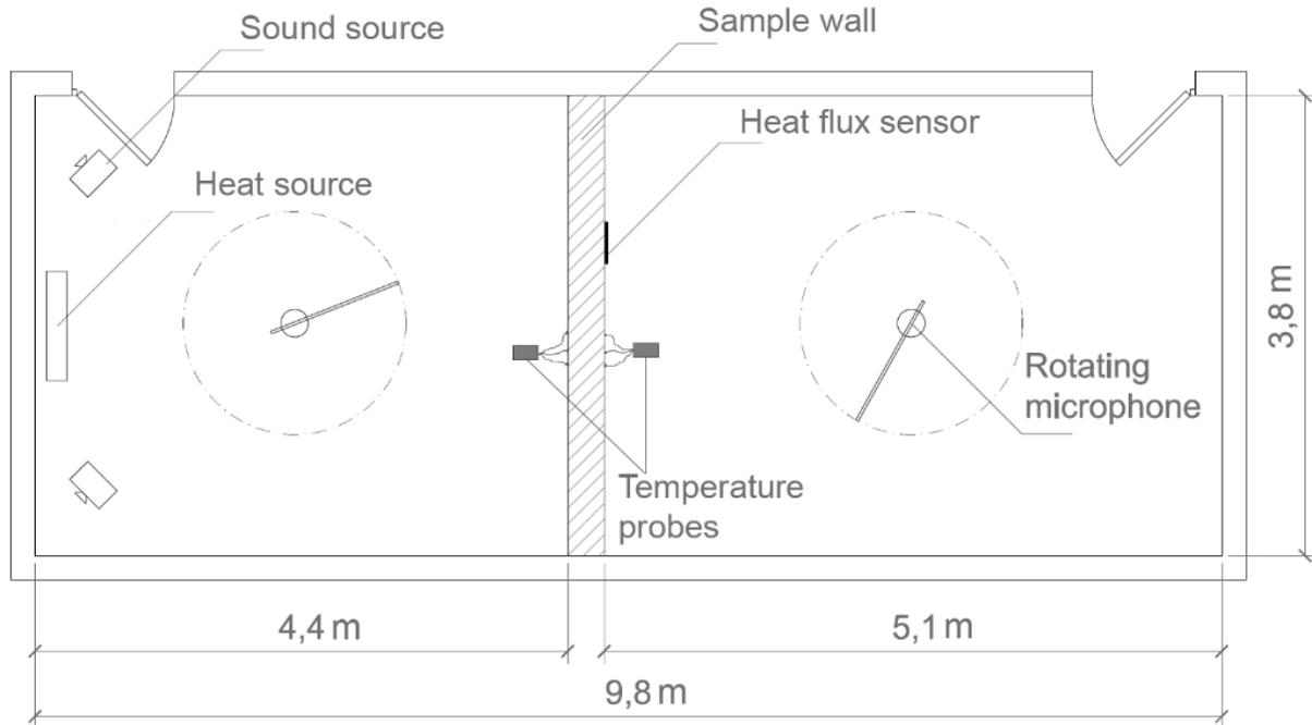
**Figure 3.6.** Transmission chamber
