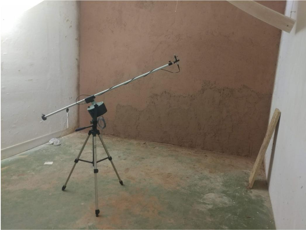
**Figure A5.** Rotating microphone inner side
