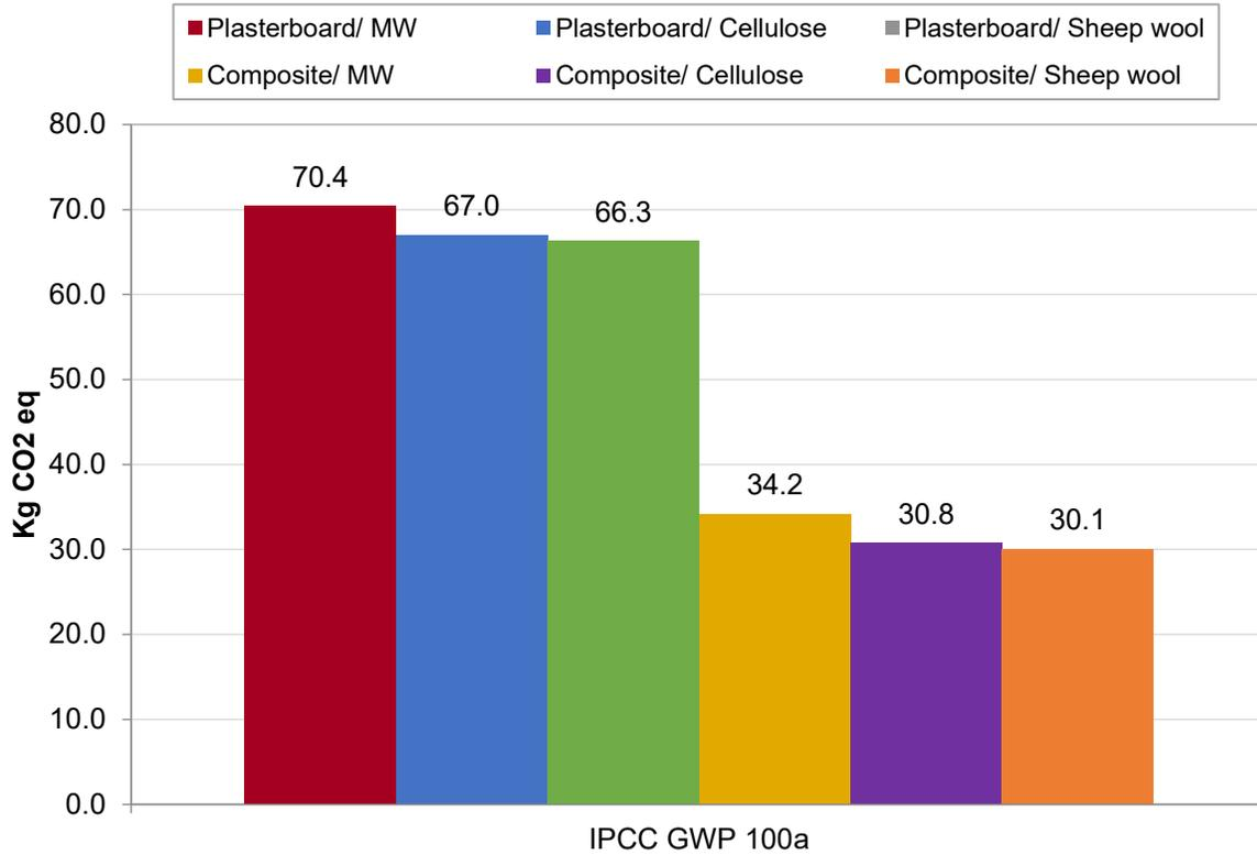
**Figure 2.4.** Carbon dioxide equivalent emitted by each typology. IPCC GWP 100a.
