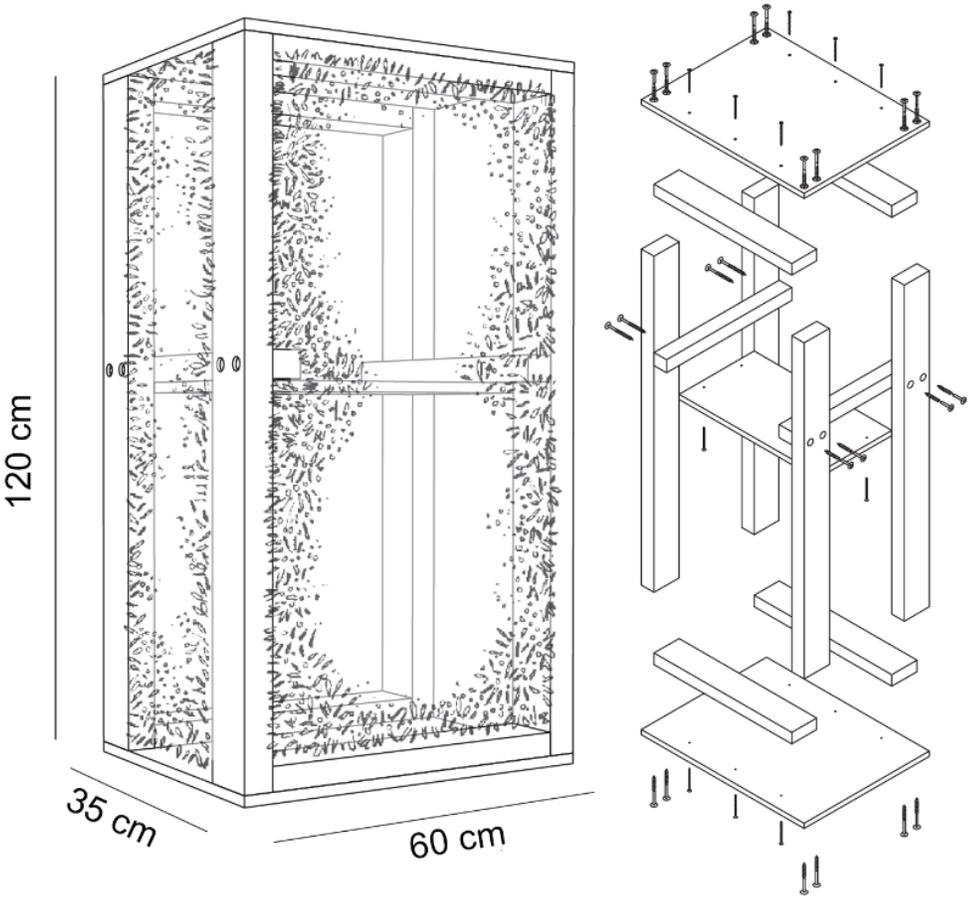
**Figure 3.3.** Straw panel dimensions and frame design
