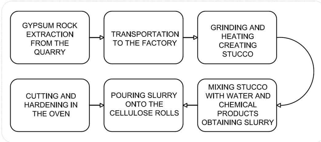
**Figure 1.1.** Plasterboard manufacturing process
