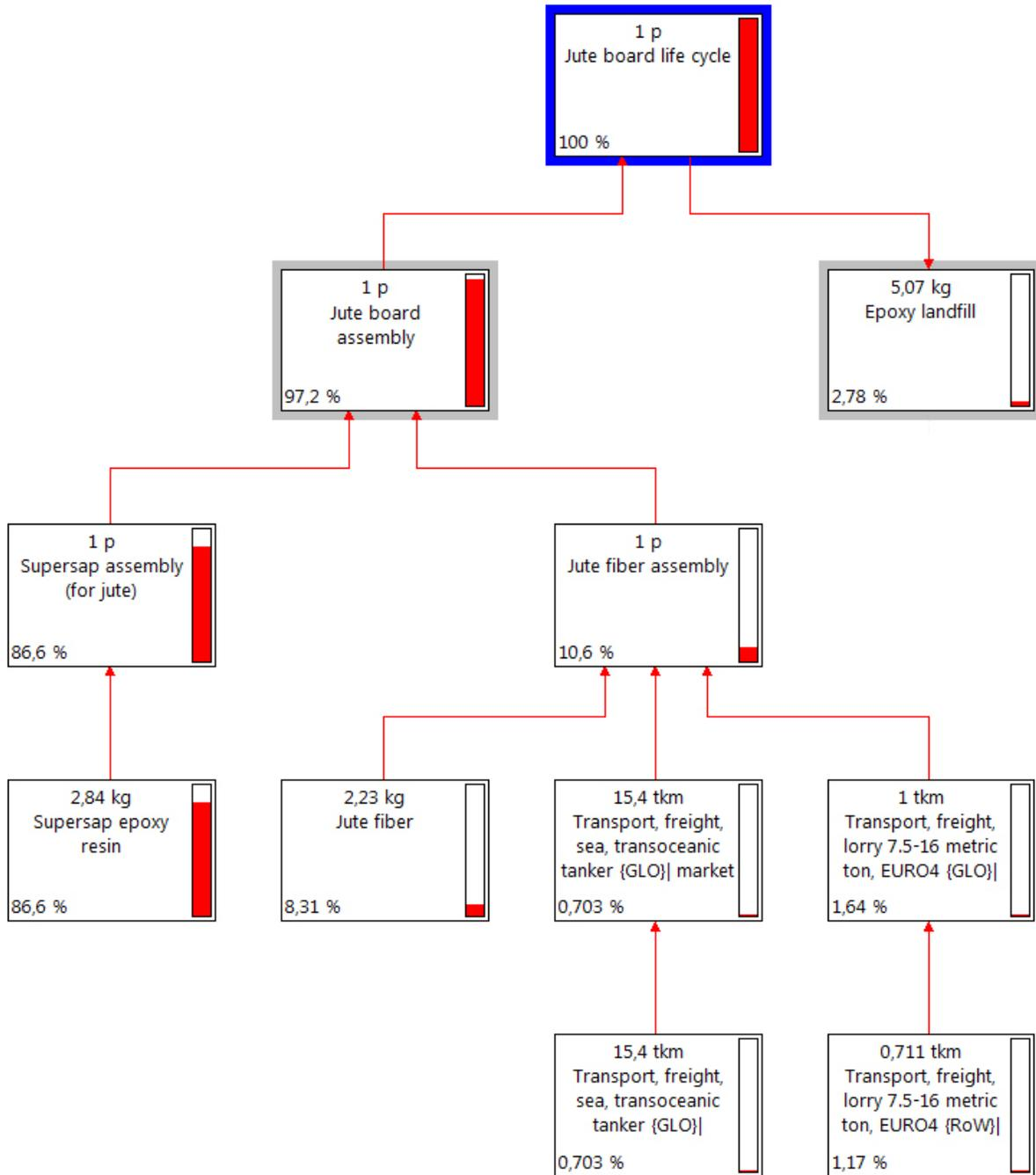
**Figure 1.7.** Network of the life cycle of the jute composite board
