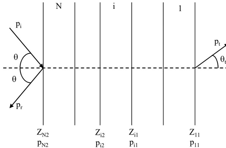
**Figure 2.2.** Ookura & Saito simulation process.  $p_t$ : transmitted pressure,  $p_i$ : incident pressure,  $p_r$ : reflected pressure,  $\theta$ : angle of incidence of the acoustic wave,  $Z$ : complex characteristic impedance.  $N$  references the number of elements. The physical parameters are numbered with the subscript  $i = 1, 2, \dots, n$  to indicate the element and a second subscript to indicate the right or the left face of the element.
