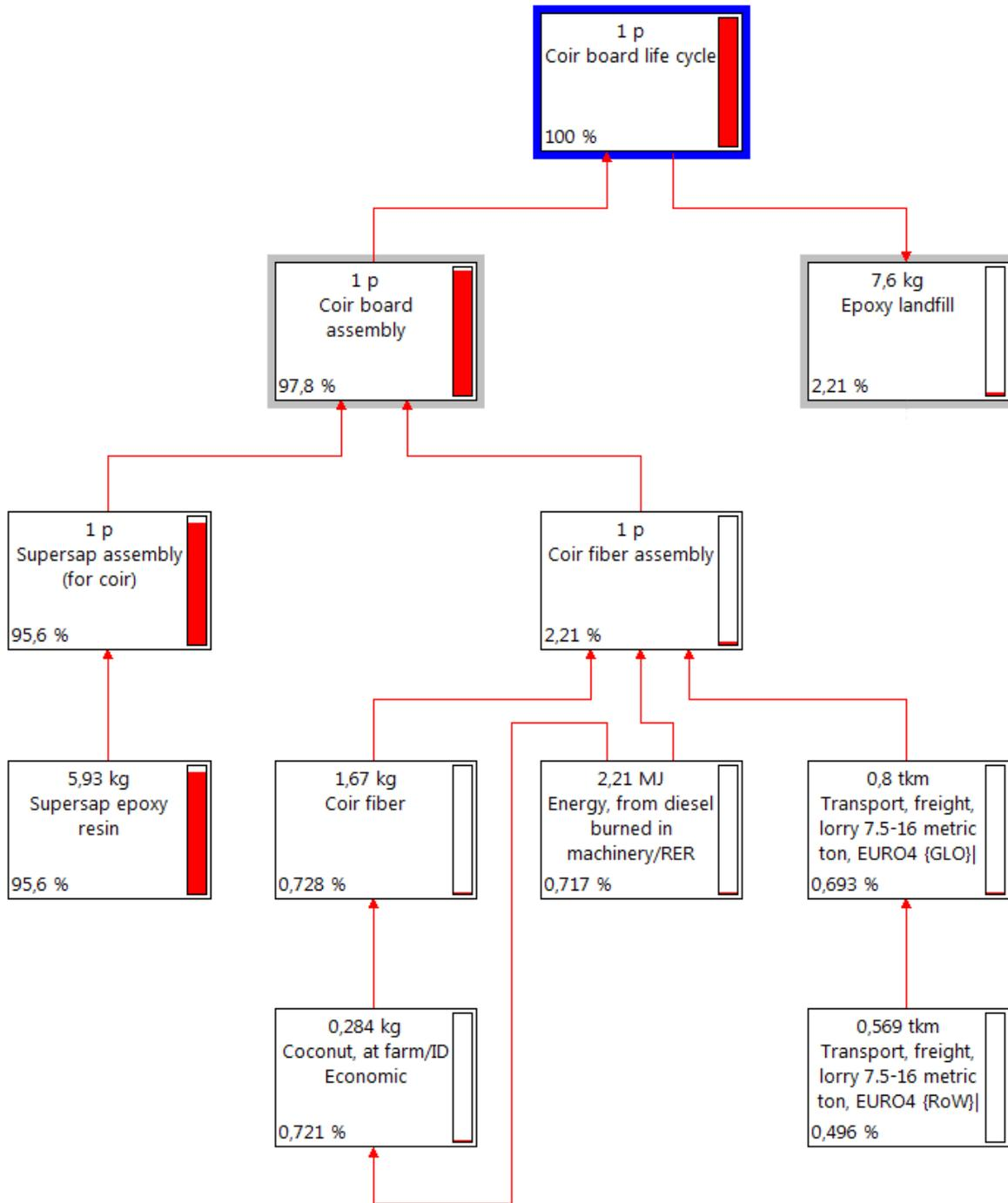
**Figure 1.9.** Network of the life cycle of the coir composite board
