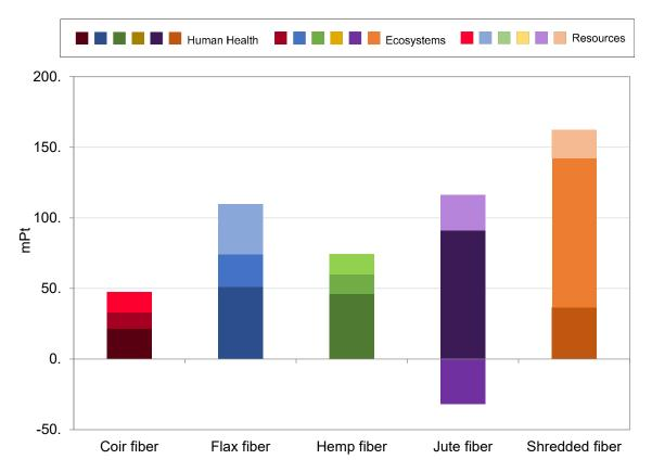
Figure 1.16 Single score result of each fiber. IPCC.GWP 100a. method. Comparative analysis of the environmental impacts produced by each fiber
