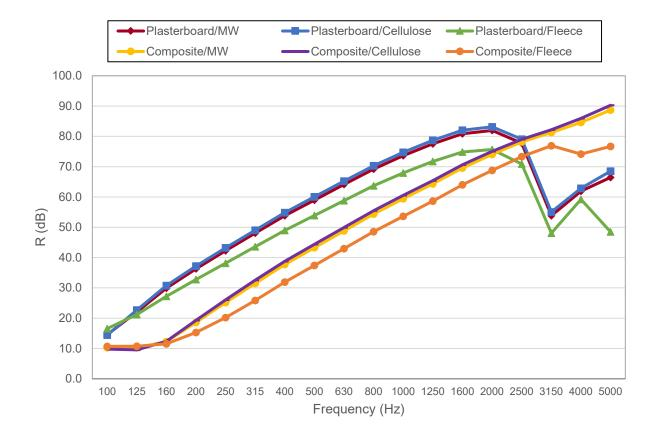
Figure 2.3. Airborne noise insulation simulation results of each typology under study.
