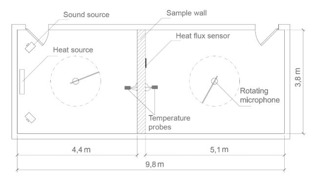
Figure 3.6. Transmission chamber
