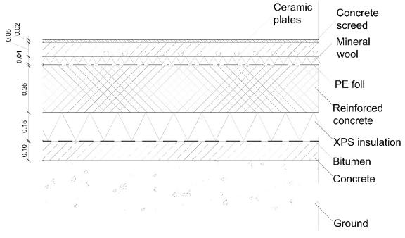
Figure D11. Section of the ground floor
