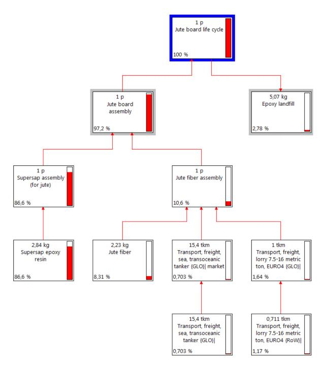
Figure 1.7. Network of the life cycle of the jute composite board
