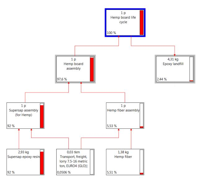
Figure 1.10. Network of the life cycle of the hemp composite board
