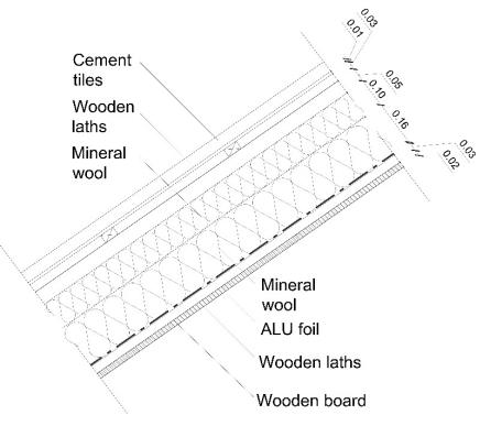
Figure D12. Section of the roof (R1)
