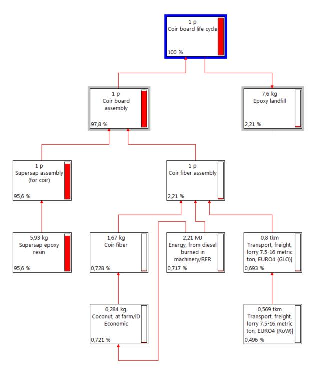
Figure 1.9. Network of the life cycle of the coir composite board
