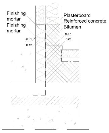
Figure D10. Section of the exterior wall ground floor bottom (W2)
