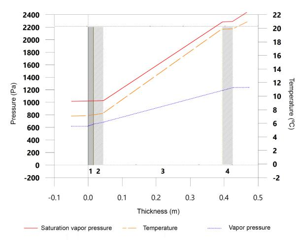
Figure 3.10. Saturation vapor pressure distribution
