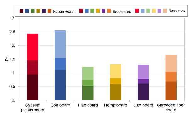
Figure 1.14. Single score result using the Recipe Endpoint (H) method. Comparative analysis of the environmental impacts produced by a 1m<sup>2</sup> board
