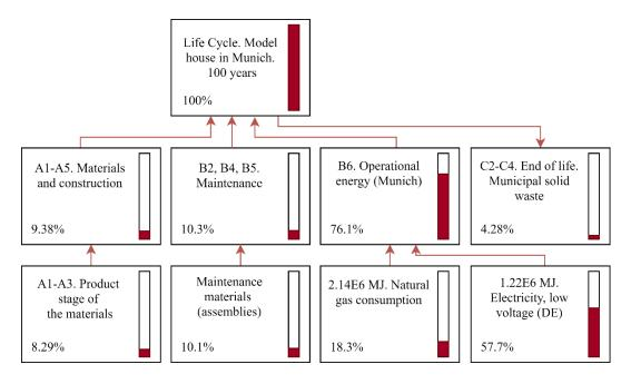
Figure 4.6. Contribution of each module to the total carbon emissions in Munich
