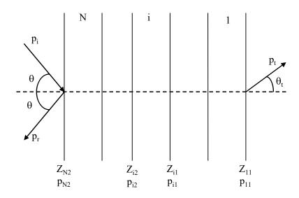
Figure 2.2. Ookura & Saito simulation process. p<sub>t</sub>: transmitted pressure, p<sub>i</sub>: incident pressure, p<sub>r</sub>: reflected pressure, θ: angle of incidence of the acoustic wave, Z: complex characteristic impedance. N references the number of elements. The physical parameters are numbered with the subscript i = 1, 2, ..., n to indicate the element and a second subscript to indicate the right or the left face of the element.
