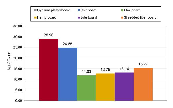
Figure 1.12. Comparative assessment of the carbon dioxide emissions by 1m<sup>2</sup> of material
