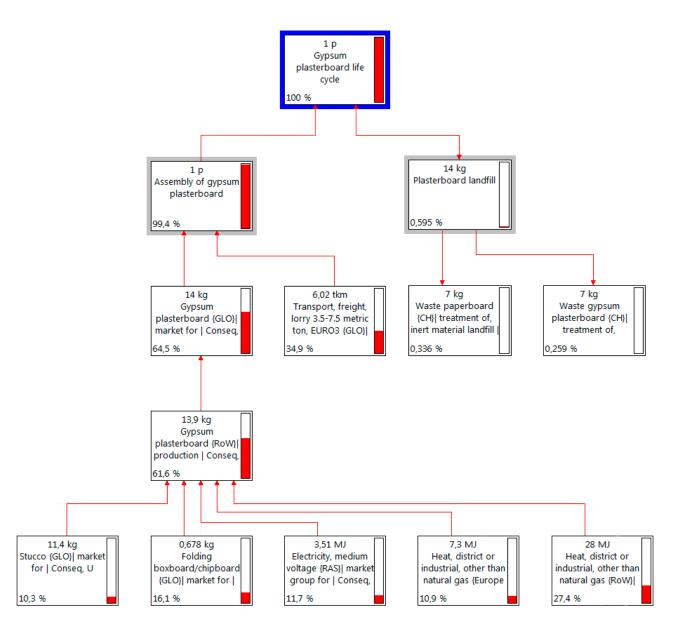
Figure 1.6. Network of the life cycle of gypsum plasterboard
