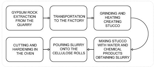
Figure 1.1. Plasterboard manufacturing process
