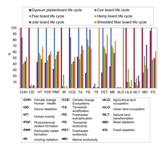
Figure 1.13. Characterization using the Recipe Endpoint (H) method. Comparative analysis of the environmental impacts produced by a 1m<sup>2</sup> board.
