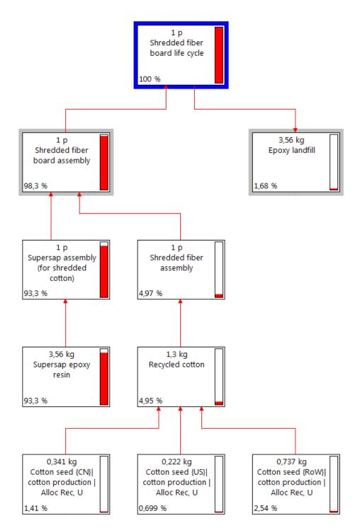
Figure 1.11. Network of the life cycle of the shredded cotton composite board
