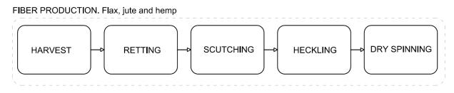
Figure 1.2. Flax, jute, and hemp manufacturing process
