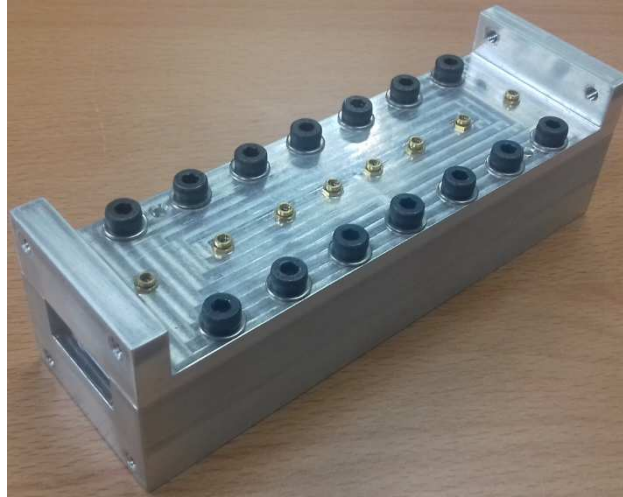
Figure 4.18: Manufactured prototype in aluminum of the in-line hybrid SIR filter with body and cover (no silver plating).
