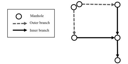
Figure 1. Types of pipes in the sewer network.
