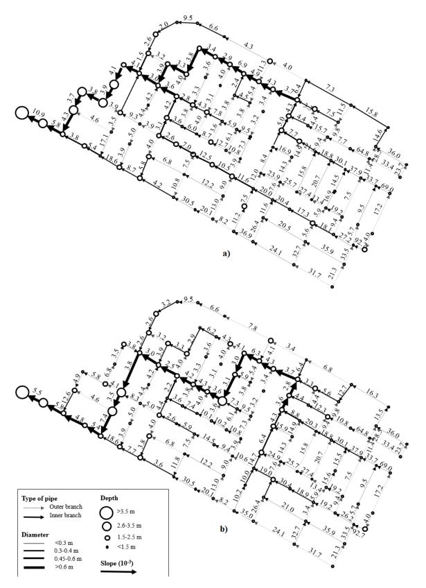
**Figure 8.** Scheme (not to scale) of the best design of the benchmark network proposed by Duque et al. [45] with (**a**) the cost function of Li and Matthew [34] and (**b**) the cost function of Maurer et al. [47].
