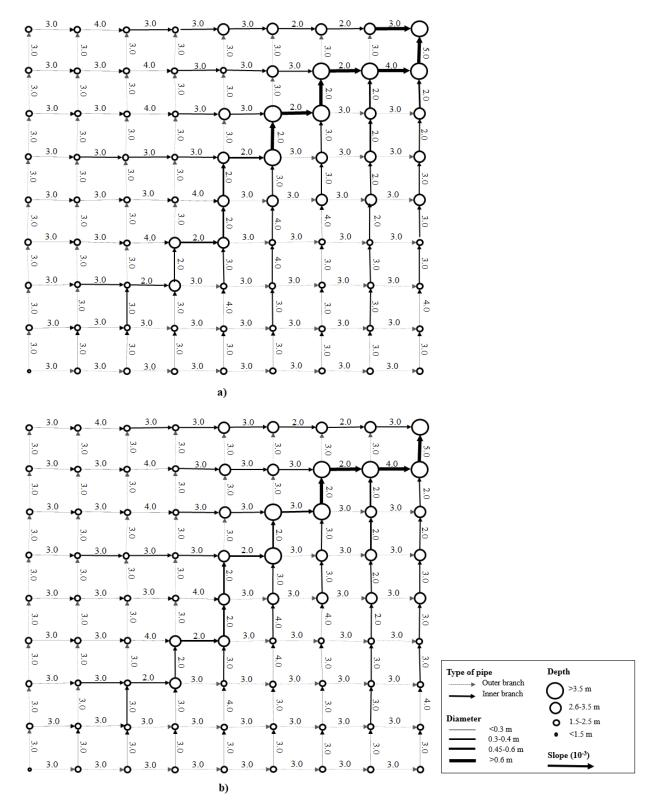
**Figure 7.** Scheme (not to scale) of the best design of the benchmark network proposed by Moeini and Afshar [46] with (a) the cost function of Li and Matthew [34] and (b) the cost function of Maurer et al. [47].
