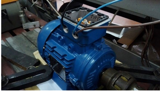
Fig. 2 – 0.55 kW, 910 rpm, 50 Hz, 2 pair of poles induction machine used for experimental tests.
