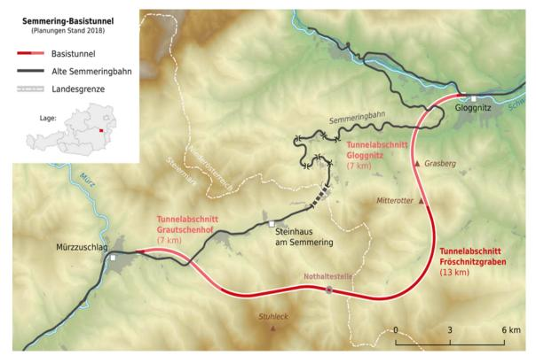
Figure 13 – Routing of the Semmeringbasis tunnel.
