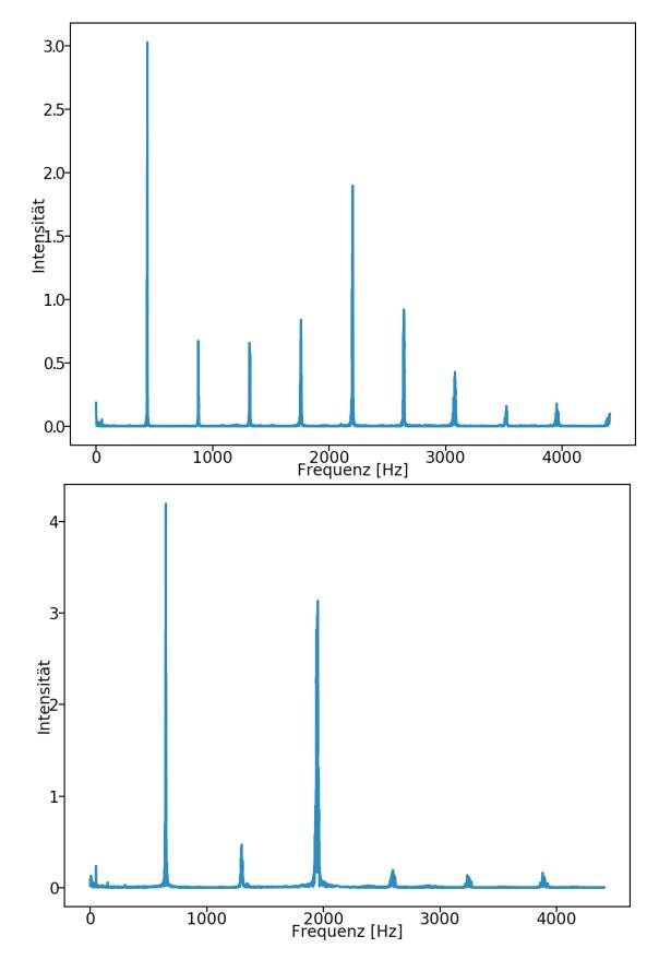
Figure 15 – Frequency spectra of two different instruments (©Patrick Capraro 2021). Up: Spectrum of a violoin. Down:Spectrum of a flute
