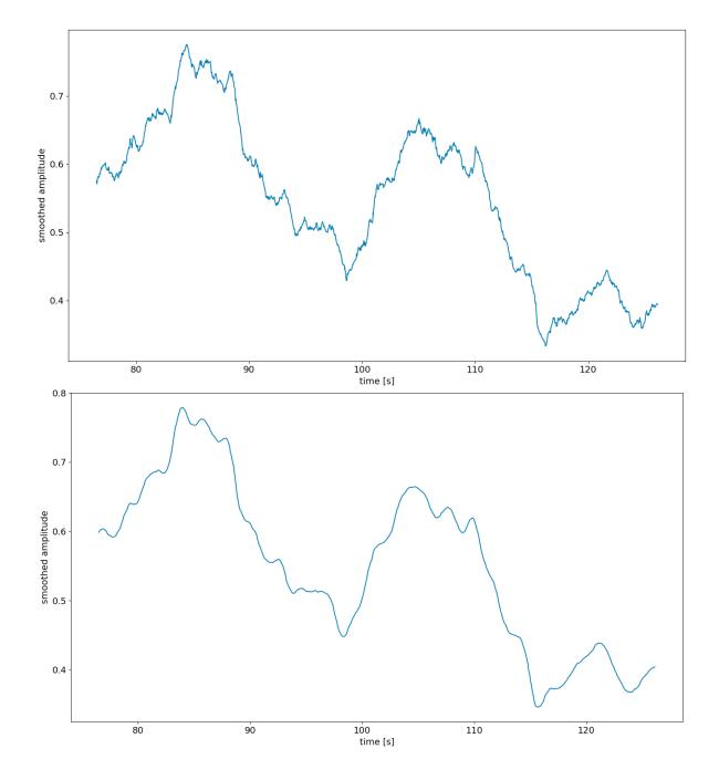
Figure 11 – First and second iteration step of the smoothing algorithm (©Patrick Capraro 2021)
