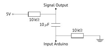
Figure 16 – Offset circuit for recording an analog audio signal (©Patrick Capraro 2021)
