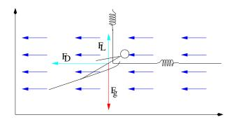
Figure 10 – Measuring lift and drag of an athlete in the air stearm of a wind channel.
