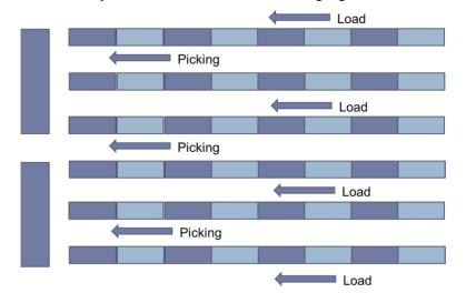
c) A system of low shelves with lockers with a total capacity of 2.000 looms
