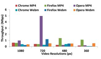
Figure 8. Throughput as a function of the video resolution on Android
