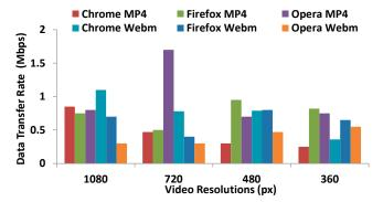
Figure 9. Data transfer rate as a function of the video resolution on Android Kit Kat
