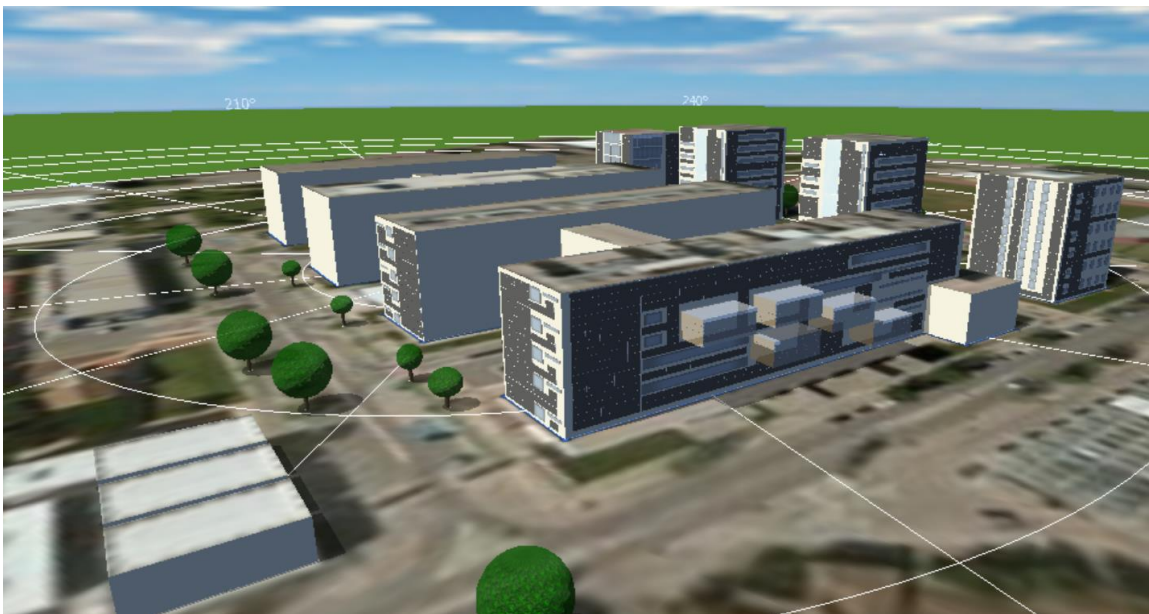
Figure 9: Possible result from a PV*SOL project
