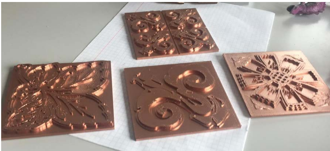
Figure 4. 3D printed models of Central Market tiles for tactile interpretation.
