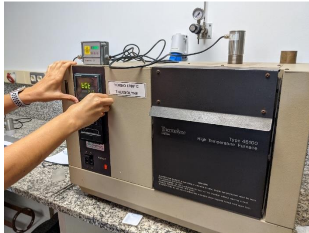
Figure 8 – Furnace used for measuring emissivity with the pyrometer on top.
