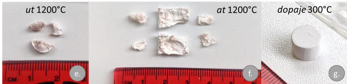
Figure 13 - Samples sintered by microwaves at high temperature and with magnetic field.
