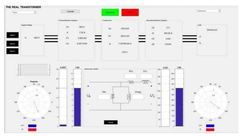
Figure 2. Shortcircuit test.
