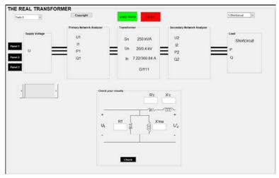
Figure 1. General view before starting the shortcircuit test.
