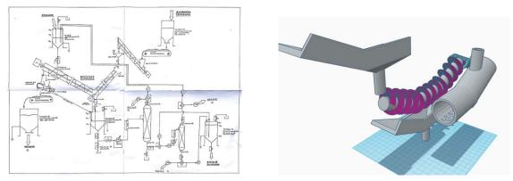
Figure 1. Example of the flow diagram of the solid-liquid extraction installation and example of a solid-liquid extractor design performed by the students of Elq3
