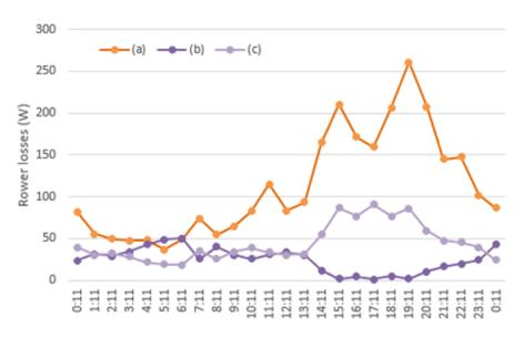
**Figure 5.** Transformer power losses in 24 h of a weekday due to: (a) active currents ( $P_{ca}$ ); (b) reactive currents with capacitors ( $P'_{cr}$ ); and (c) reactive currents without capacitors ( $P_{cr}$ ).
