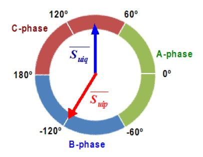
**Figure 2.** Representation of the vector unbalanced power components:  $S_{uip}$  (red vector) and  $S_{uiq}$  (blue vector).
