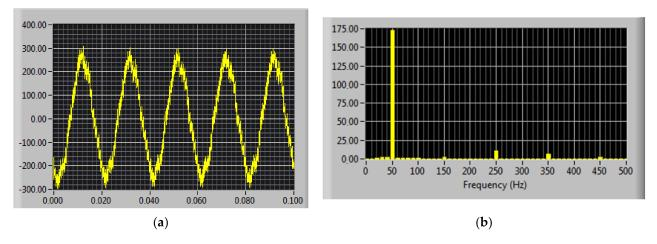
Figure 13. Current flowing through the A-phase of transformer at 16:11 on a working day: (a) waveforms; (b) harmonic diagram.
