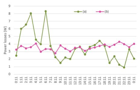
**Figure 8.** Transformer power losses in 24 h of a holiday caused by: (a) unbalanced currents ( $P_{cu}$ ) and (b) distorted currents ( $P_{ch}$ ).
