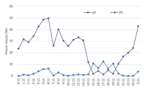
**Figure 11.** Transformer power losses, on weekdays, due to: (**a**) actual reactive currents with non-optimized capacitors; and (**b**) reactive currents with capacitor banks optimized.
