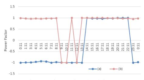
**Figure 10.** Transformer power factor (PF) after applying the first optimization procedure on the capacitor banks: (**a**) weekdays (disconnecting  $Q_{c1}$ ); (**b**) holidays (disconnecting  $Q_{c2}$ ).
