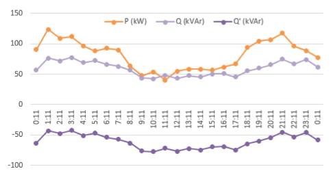
**Figure 4.** Powers delivered by the transformer in 24 h of a holiday: active P(kW) and reactive Q'(kVAr) powers registered by the Fluke 435 Series II; and reactive power supplied with no capacitor banks Q (kVAr) (a negative sign indicates capacitive reactive powers).
