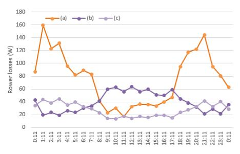
**Figure 6.** Transformer power losses in 24 h of a holiday due to: (**a**) active currents ( $P_{ca}$ ); (**b**) reactive currents with capacitors ( $P'_{cr}$ ); and (**c**) reactive currents without capacitors ( $P_{cr}$ ).
