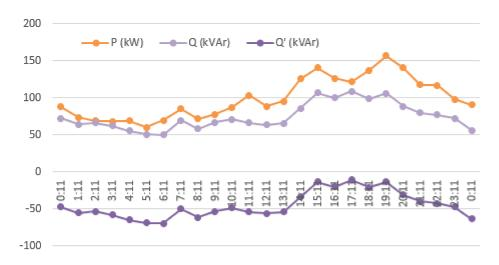
**Figure 3.** Powers delivered by the transformer in 24 h of a weekday: active P(kW) and reactive power Q'(kVAr), registered by the Fluke 435 Series II; and reactive power supplied with no capacitor banks Q(kVAr) (a negative sign indicates capacitive reactive powers).
