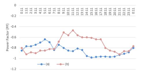
**Figure 9.** Transformer power factor (PF) on: (**a**) weekdays; and (**b**) holidays (positive values indicate inductive PF, whereas negative values mean capacitive PF).
