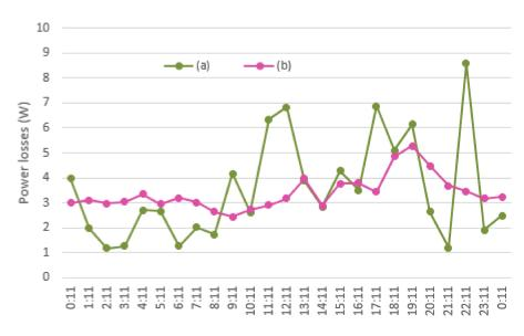
**Figure 7.** Transformer power losses in 24 h of a weekday caused by: (**a**) unbalanced currents ( $P_{cu}$ ) and (**b**) distorted currents ( $P_{ch}$ ).
