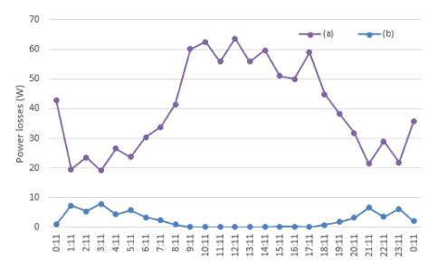
**Figure 12.** Transformer power losses, on holidays, due to: (**a**) actual reactive currents with non-optimized capacitors; and (**b**) reactive currents with capacitors optimized.
