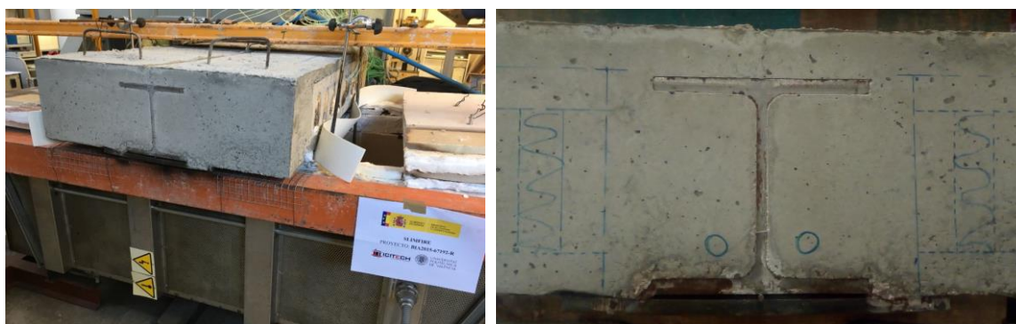
Figure 13: Experimental setup for elevated temperature slim-floor tests at UPV, Valencia (Spain) [42]
