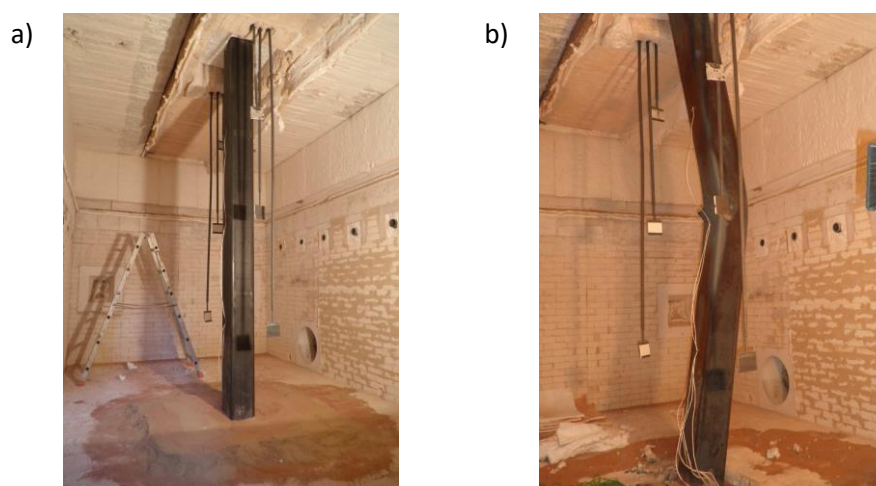
Figure 3: View of a square CSFT column before (a) and after (b) the fire test [6]
