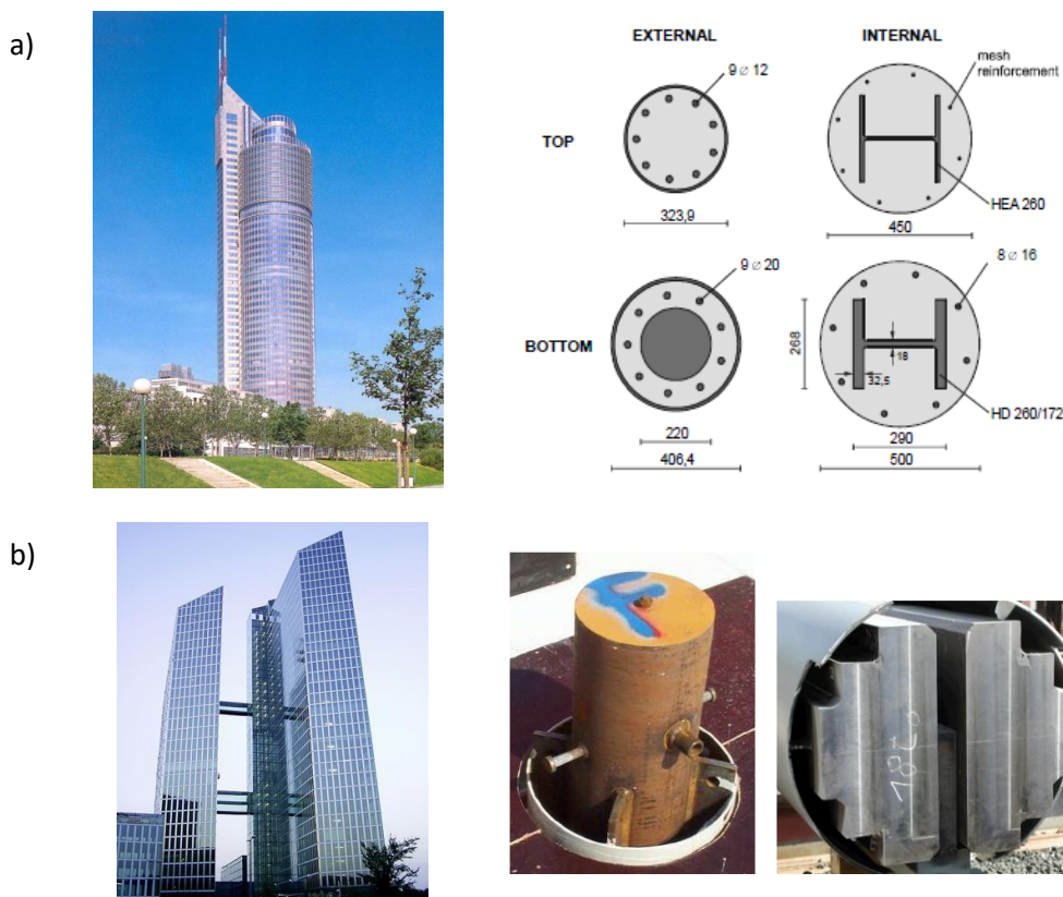
Figure 6: Examples of buildings using innovative composite columns: a) Millennium Tower (Wien, Austria), b) Highlight Towers (Munich, Germany) [6]
