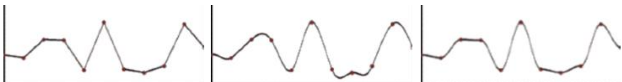
Figure 7 Comparison of the linear (left) cubic (middle) and cosine (right) interpolation (Aran D.).
