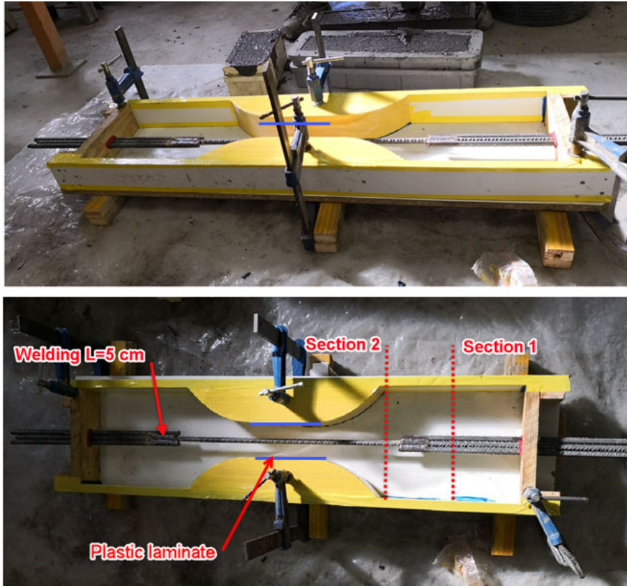
Figure2. Dog bone-shaped specimen and reinforcement detail
