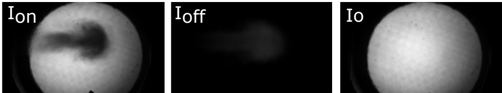
Figure 3.25: Light intensity of frame with LED-on (left), LED-off (center), and background before the start of injection(right).
