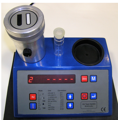
Figure 6.27. Experimental setup to analyse the insoluble content in engine oils.
