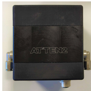
Figure 3.74. Particle counting analyser devices to obtain ISO codes of wear metals in lubricants.
