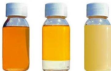
Figure 3.59. Water in oil phases: dissolved (minor level), free (overloaded level) and emulsified (major level).
