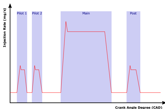
Figure 6.69. Common injection setup comprising four injections: pilot 1, pilot 2, main and post injection.
