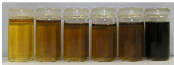
Figure 6.45. Picture of a set of low-mileage samples, where it can be see the evolution of the oil colouring to blacker tones as the oil accumulates use: 0, 15, 30, 45, 60 and 240 minutes (from left to right).
