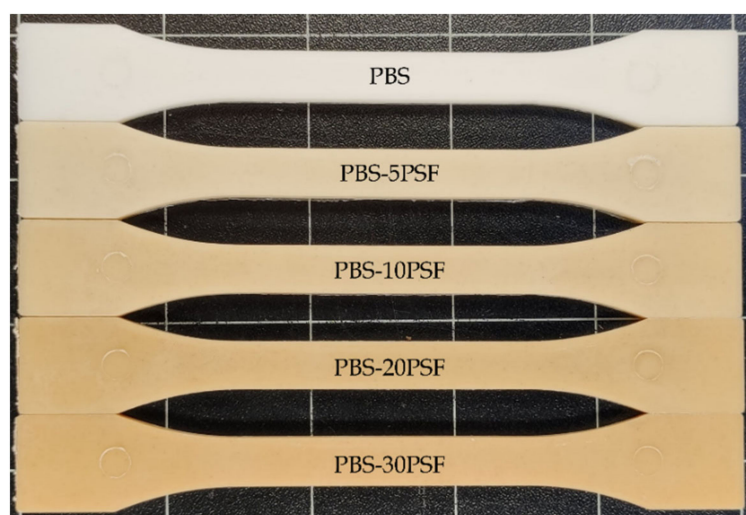
Figure 2. Visual appearance of the injection-molded pieces of poly(butylene succinate) (PBS)/pistachio shell flour (PSF) compatibilized with poly(butylene succinate) grafted with maleic anhydride (PBS-g-MAH).
