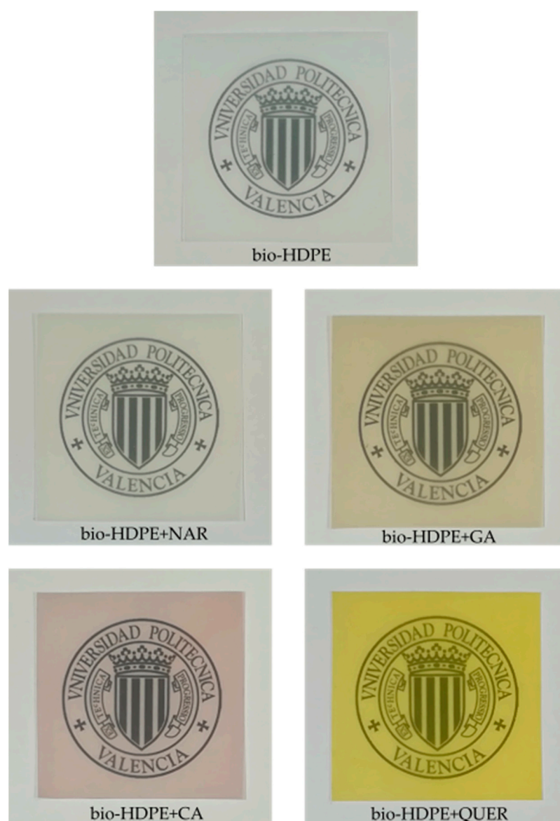
Figure 2. Visual appearance of the thermo-compressed bio-based high-density polyethylene (bio-HDPE) films containing naringin (NAR), gallic acid (GA), caffeic acid (CA), and quercetin (QUER).
