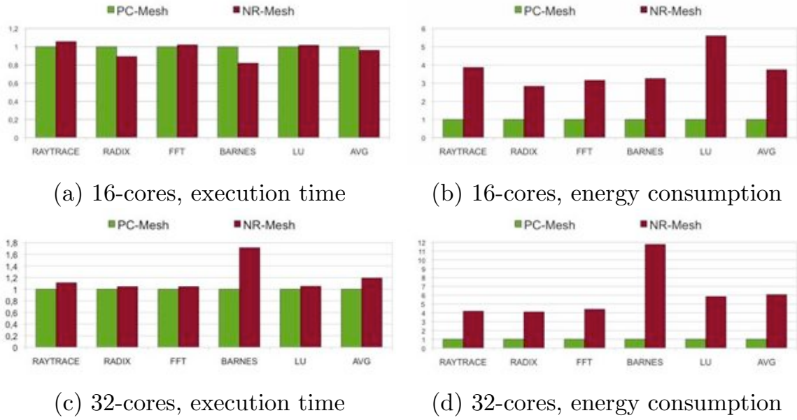
Figure 4.14: Normalized application execution time and normalized network energy consumption comparison between NR- and PC-Mesh topologies using real applications.
