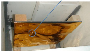
(b) Multi-Layer insulation as DUT. A rivet area is spotted.
