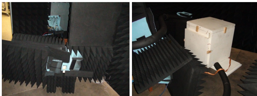
(a) Part inside the anechoic chamber - horn antennas. The multiplexer is covered by RAM absorbers. (b) Part inside the anechoic chamber - RF transparent box to accommodate the DUT during the thermal cycle tests.
