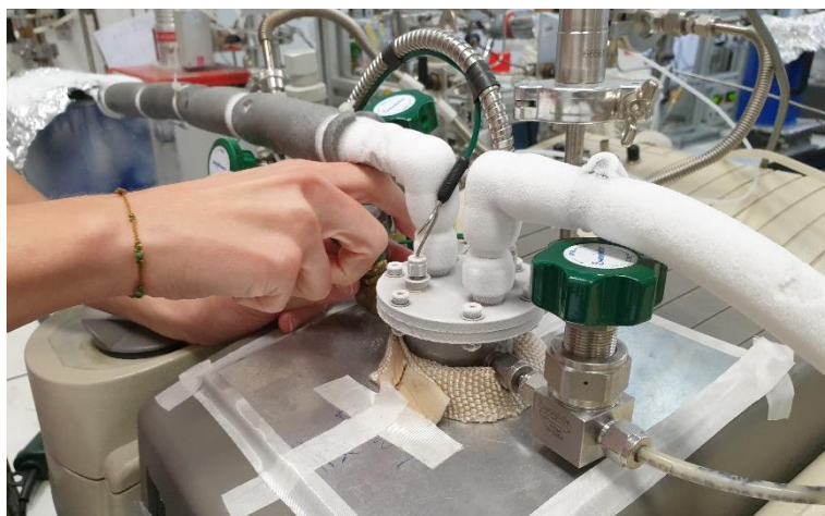
Dosing CO at -170 °C by cooling down with liquid N 2 in a catalytic cell coupled to a Thermo Nicolet Nexus IR spectrophotometer
