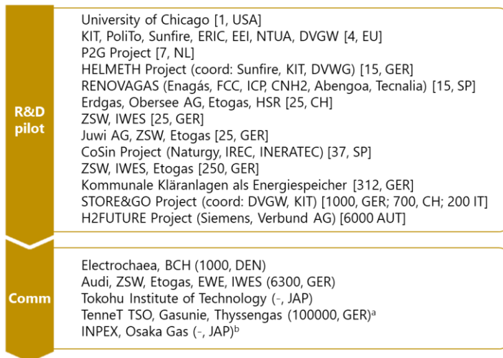
Figure 1.15 CO 2 methanation projects under different stages of development. Numbers in brackets refer to the capacity/power of the plant, expressed in kW. a First module will go into operation in 2022, full capacity in 2028. b This plant will start operations in 2024. Author credits: Cored, J.; No copyright intended.
