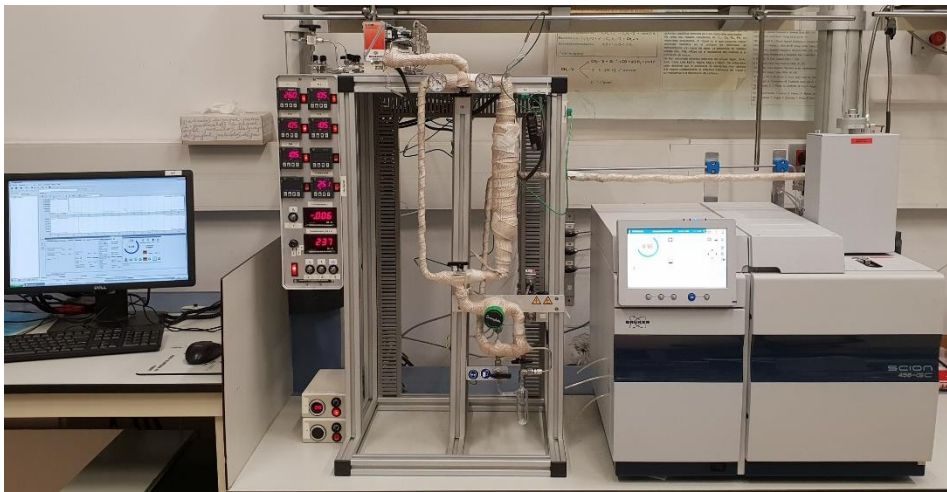
Stainless steel fixed-bed reactor setup (1-20 bar)
