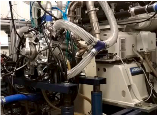
Fig. 2. Engine test bench with the 2S-ROPE fully instrumented for the experimental campaign.
