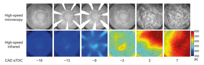
**Figure 15.** High-speed optical microscopy (**top row**) compared to high-speed infrared imaging (**bottom row**), showing the temperature distribution across the nozzle surface, as well as the radiometric temperature of the fuel sprays. Both test cases were taken using a DFI 1.3 injector under the same engine operating parameters (fuel: CEC RF-79-07; injection: 40 MPa at  $-18^{\circ}$  CA aTDC; ICP at injection: 3.1 MPa; peak motored ICP: 4.9 MPa).
