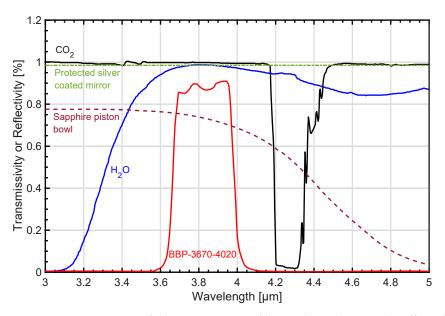
**Figure 1.** Transmissivity of the BBP-3670-4020 filter used to eliminate the effect of water and CO<sub>2</sub> absorption on the radiometric temperature.
