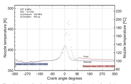
**Figure 13.** As expected, combustion results in a significant increase in peak nozzle tip temperature when compared to motored conditions. In this test point the nozzle reaches 470 K, with a temperature rise persisting through to the next TDC event (as shown in Figure 10). The test point shown here used n-dodecane injections and a swirl factor of 1.38.
