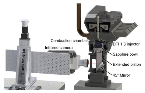
**Figure 2.** Optical engine set-up depicting the position of the injector, sapphire bowl, silver mirror and camera with respect to the test-bed. A red arrow highlights the path of the IR radiation from the injector to the camera.
