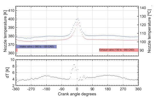
**Figure 11.** Increasing the intake gas temperature by 7 K from 318 K (red dots) to 325 K (blue dots) leads to a similar increase in nozzle tip temperature (dT = +5.5 K) towards the end of the intake stroke ( $-180^{\circ}$  CA aTDC), which indicates that the high-speed infrared thermometry is able to detect such small changes in operating conditions. The test points are motored (no fuel injection) with a swirl factor of 1.38.
