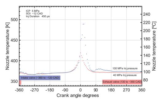
**Figure 14.** Increasing injection pressure (with injection pulse duration remaining constant) results in an increase in nozzle tip temperature, as expected. This test point nozzle tip temperature reaches 420 K and 490 K at 40 MPa and 100 MPa, respectively. These temperatures would be expected to slightly increase over time due to a carryover of temperature into the next cycles as shown in Figure 10b. The test points shown in this figure used n-dodecane injections and a swirl factor of 1.38.
