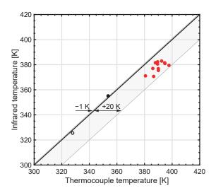
**Figure 9.** Uncertainty of measurements shows the effect of fouling on the bow ditch piston bowl. Closed symbols indicate optically fouled conditions under static (black) and motored (red) engine conditions. Open black symbols indicate static test cases with no optical fouling (cleaned optics).
