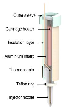
**Figure 5.** A diagram of the dummy injector nozzle used to calibrate the radiometric temperature. Within the cross section the positions of the heater cartridge, thermocouple and aluminium insert can be seen. Thermal transfer to the test-bed is reduced through the insulation layer and Teflon ring.
