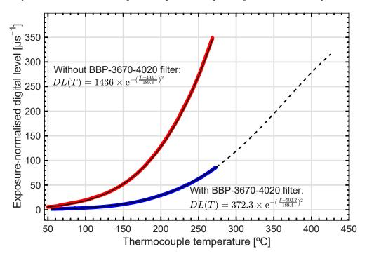
**Figure 6.** Average DL/µs values from the ROIs in the calibration images, plotted against their corresponding thermocouple values using the in-engine dummy injector nozzle. The extrapolated exponential fits were validated (Section 3.4) and then used to convert the measured radiometric temperatures into actual surface temperatures.
