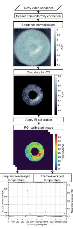
in Figure 8. The time-averaged infrared temperature was then plotted along with the instrumented injector's reading to evaluate the validity of the method.
