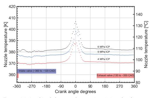
**Figure 12.** A rise in peak in-cylinder pressure shows a consistent rise in nozzle surface temperature at each 1 MPa interval. These test points were taken under motored conditions with a swirl factor of 1.38.
