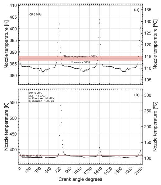
**Figure 10.** Validation of methodology across motored (**a**) and fired (**b**) test conditions, showing an excellent agreement between the mean IR and thermocouple measurements.
