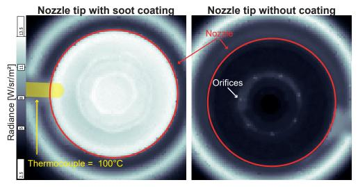
**Figure 4.** A comparison of the infrared radiation emitted by sooted (**left**) and clean (**right**) injector nozzles, heated to 100 °C. The position of the nozzle periphery is overlaid, along with the thermocouple applied onto the nozzle surface to measure the actual surface temperature.
