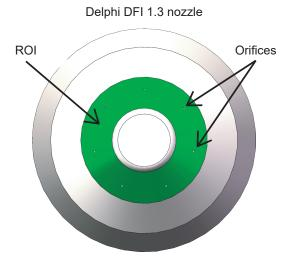
**Figure 7.** A schematic of the DFI 1.3 injector nozzle used in these analyses. The region of interest for the investigations presented is demonstrated by the green highlighted area on the inclined plane where the nozzle offices are placed on.
