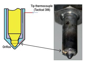
**Figure 3.** Diagram and photograph of the thermocouple-instrumented injector nozzle. A thermocouple was embedded at the injector tip, near the orifices, to provide time-averaged nozzle surface temperature.
