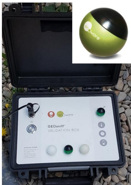
Figure 2. The GEOsniff Validation Box with two GEOsniff sensors (green/black balls) and two blind balls (white), which are for checking the recoverability of the real sensors.
