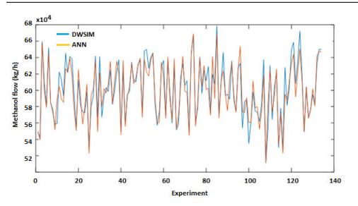
Figure 9. Comparative graph of the experimental data (DWSIM) and ANN predictions regarding methanol flux (kg/h).
