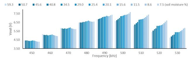
Figure 32. The Vout in the different frequencies tested in the prototype NP4.
