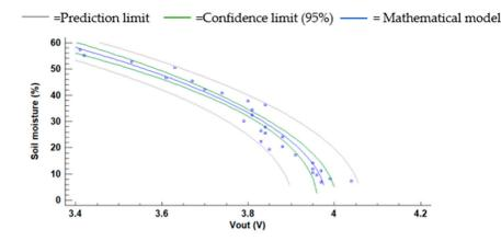
Figure 24. The Vout of prototype NP1 frequency 750 kHz.
