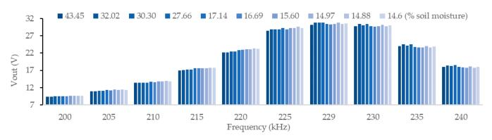
a correct behavior for high moisture at the 229 kHz frequency and low moisture at the 225 kHz frequency.
