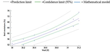
Figure 17. Vout of P5 using S1 and its mathematical model.
