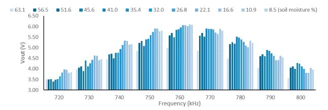
Figure 30. The Vout in the different frequencies tested in prototype NP3.
