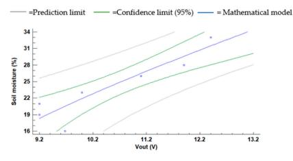
Figure 22. Vout of P8 using S5 and its mathematical model.
