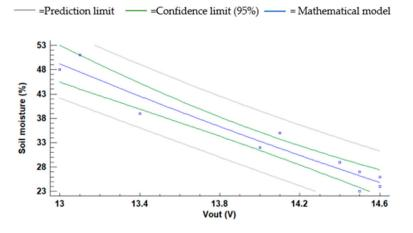
Figure 20. Vout of P8 using S3 and its mathematical model.
