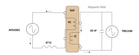
Figure 3. Electric circuit of the sensor.
