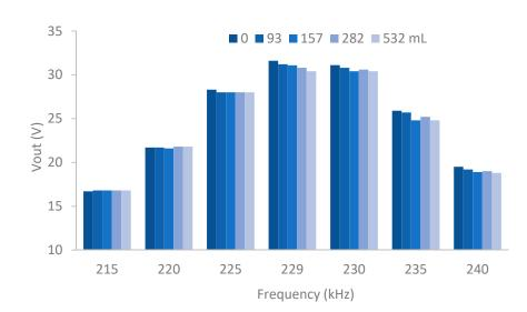
Figure 8. Vout of P5 using samples with different water content.
