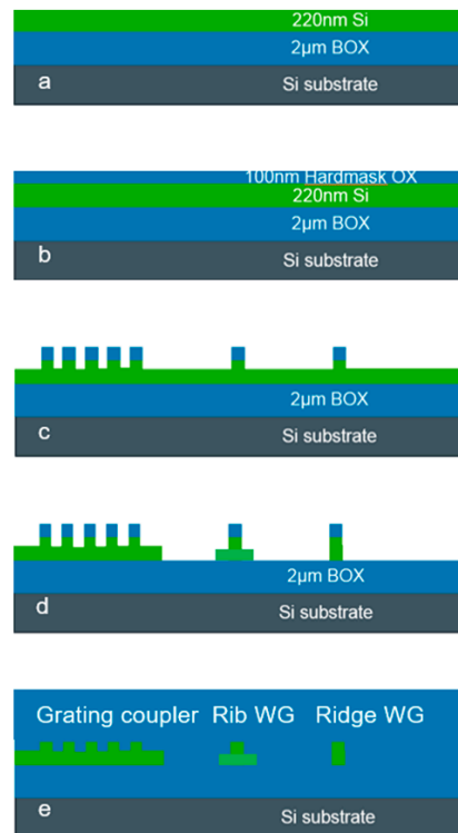
Figure 6. Passive device manufacturing. Schematic representation of the main process steps: (a) SOI wafer as starting material, (b) silicon dioxide hard mask deposition, (c) silicon structuring by time-controlled shallow etching, (d) complete silicon etching in selected areas, (e) silicon dioxide top cladding deposition with Chemical-mechanical polishing (CMP) planarization.
