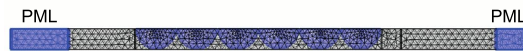
Figure 4. Top view of the numerical domain, exhibiting the tetrahedra elements, Perfectly Matched Layers (PML) locations, and the quarter spheres.
