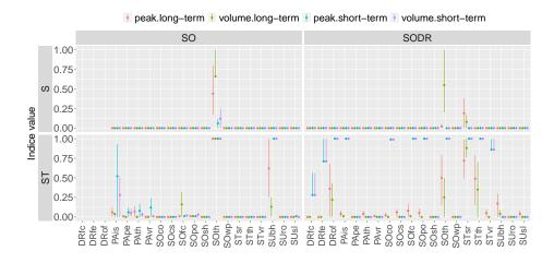
Figure 5: Estimated total (ST) and first-order (S) effects with their confidence intervals for scenarios excluding (SO), on the left, and including (SODR), on the right, the effects of drain. Different colours are shown for scenarios considering the long- or short-term modelling and measuring outflow peak or volume).
