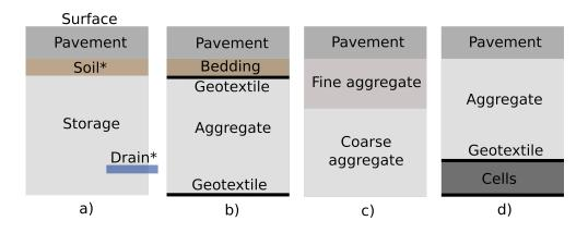
Figure 1: PP cross-sections (a) as defined in the SWMM model (b) with bedding layer and geotextiles, (c) various aggregate types, and (d) cells below aggregate with geotextiles.
