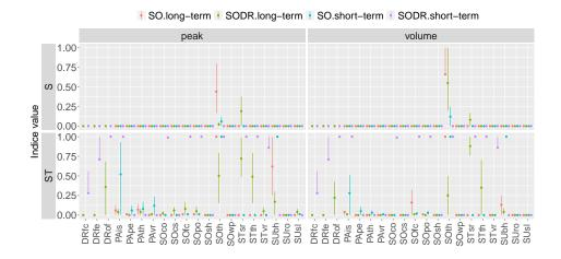
Figure 6: Estimated total (ST) and first-order (S) effects with their confidence intervals for scenarios measuring outflow peak (left) and outflow volume (right). Different colours are shown for scenarios including (SODR) and excluding (SO) the effects of drain and considering the short- or long-term modelling.
