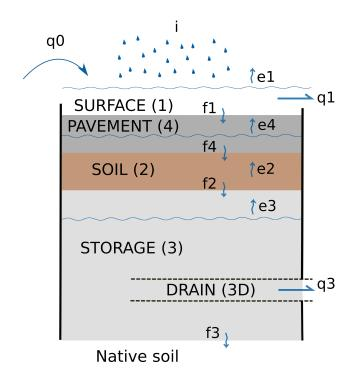
Figure 2: SWMM layers and flux terms for PP.
