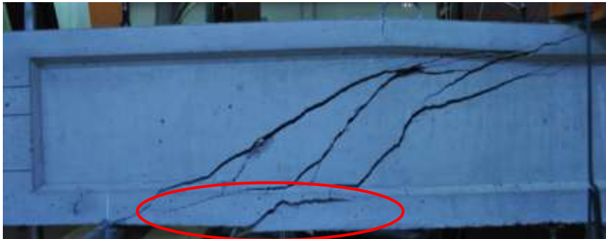
Fig. 6. 14 Small cover of beam M-0.
