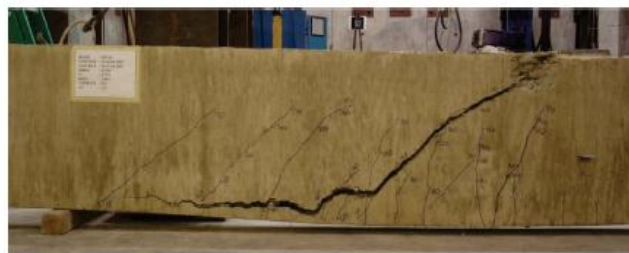
(b) Shear compression failure in FRC beam
