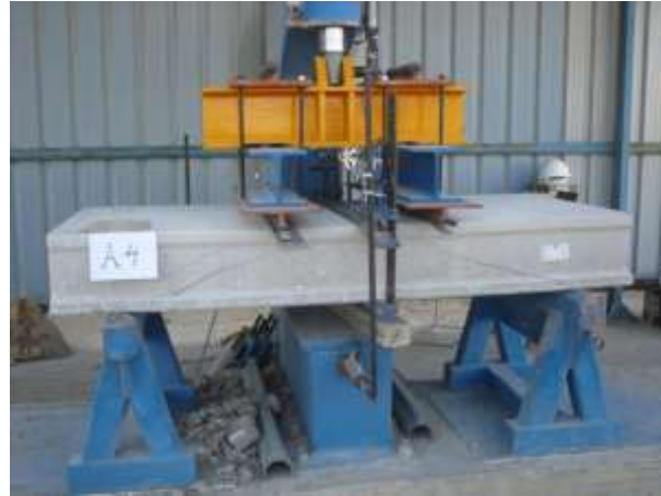
Fig.7. 5 Test set-up. Shear diagonal tension failure
