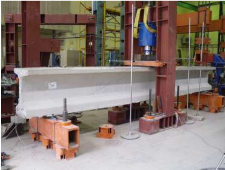
Fig.4. 5 Beam during shear test
