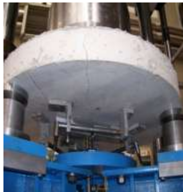
Fig.5.7 Round panel during the test
