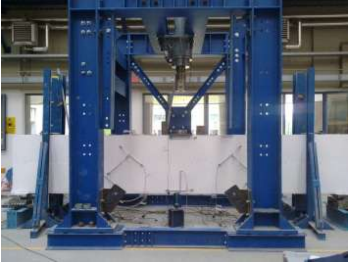
Fig.5.14 Front view of a beam H1000 under preparation for the test
