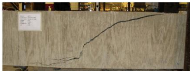
(c) Diagonal tension failure in RC beam without stirrups
