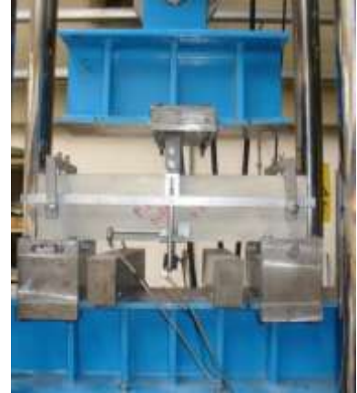
Fig.5.5 Prismatic specimen during the flexural tensile strength test according to EN 14651
