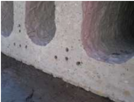
Fig.7. 9 Sliding of the strands in concrete
