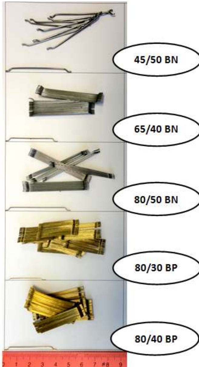
Fig.6. 1 Typology of steel fibers used in this experimental program (scale lines indicate millimeters)
