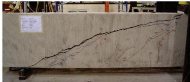
(a) Diagonal tension failure in FRC beam
