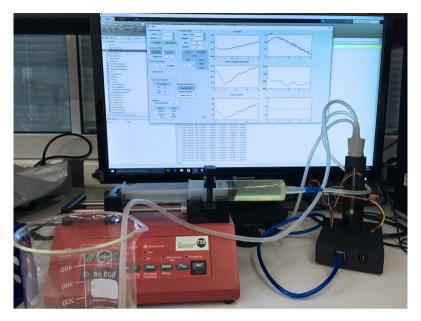
Figure 6.8: Experimental turbidostat setup.
