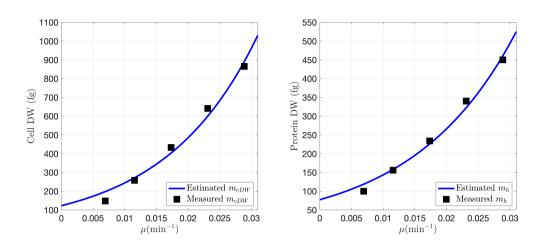
**Figure A.4:** Fit between the cell dry weight (left) and the protein content dry weight (right) as a function of the specific growth rate using the expressions (A.65) and (A.66) respectively.
