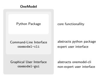
**Figure 3.2:** Internal structure of *OneModel*, where its core is a *Python* package. The command-line interface abstracts the functionality of the python package, and the graphical user interface represents the functionality of the command-line interface.
