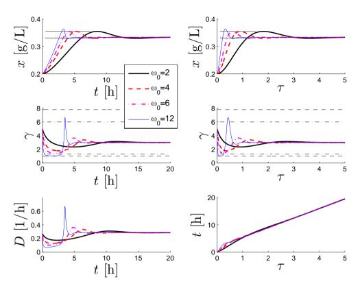
**Figure 6.3:** Set-point change for Haldane kinetics. Former set-point:  $(x_0, s_0, \gamma_0) = (.2, 3.16, 5)$ , new set-point:  $(x^*, s^*, \gamma^*) = (1/3, 2.86, 3)$ .
