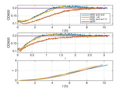
**Figure 6.9:** Biomass concentration x in the t time scale (top), in the transformed  $\tau$ -time (middle), and relationship between t and  $\tau$ (bottom). Initial conditions:  $x_0 \approx 0.12(OD_{600})$ . Set-point  $x^* = 0.2$ . Proposed controller: (a, b) = (4, 7.11) (yellow), (a, b) = (2, 4) (blue). Baseline controller (orange).
