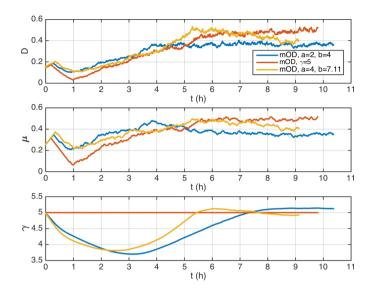
**Figure 6.10:** Dillution D (top), estimated specific growth rate  $\mu$  (middle) and controller gain  $\gamma$  (bottom). Proposed controller: (a, b) = (4, 7.11) (yellow), (a, b) = (2, 4) (blue). Baseline controller (orange).
