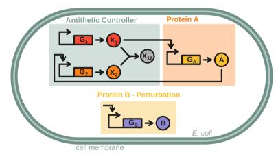
Figure 5.1: The schematic representation of the antithetic controller regulating the expression of protein A and, independently, the expression of protein B causing a perturbation in the host cell.
