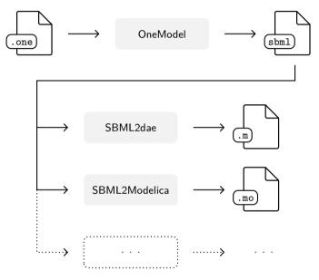
**Figure 3.1:** OneModel workflow. The user writes a model using OneModel syntax (".one"). Then, the model is exported into SBML using OneModel. Finally, the SBML-compliant tools can be used as (i) SBML2dae generates a Matlab implementation of the model (".m"), or (ii) SBML2Modelica [67] generates a Modelica representation (".mo").
