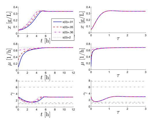
Figure 6.6: Process start-up from different initial substrate concentrations for Monod kinetics. Initial condition:  $(x_0, s_0, \gamma_0) = (.05, s_0, 3)$ , set-point:  $(x^*, s^*, \gamma^*) = (1/3, 2.86, 3)$ . Controller tuning:  $(\xi, \sigma) = (.75, 3)$ .
