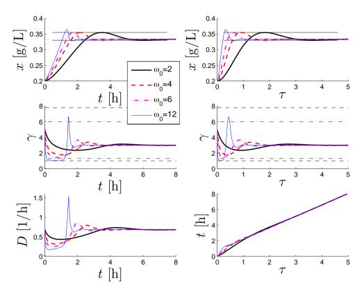
**Figure 6.2:** Set-point change for Monod kinetics. Former set-point:  $(x_0, s_0, \gamma_0) = (.2, 3.16, 5)$ , new set-point:  $(x^*, s^*, \gamma^*) = (1/3, 2.86, 3)$ .
