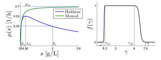
**Figure 6.1:** (a) Specific growth kinetics  $\mu(s)$ . (b) Bounding function  $f(\gamma)$  of controller (6.15).
