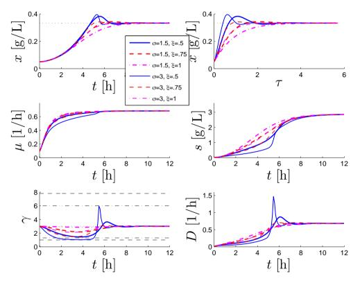
**Figure 6.4:** Process start-up for Monod kinetics. Initial condition:  $(x_0, s_0, \gamma_0) = (.05, .01, 3)$ , set-point:  $(x^*, s^*, \gamma^*) = (1/3, 2.86, 3)$ .
