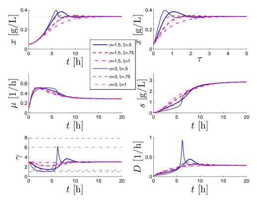
**Figure 6.5:** Process start-up for Haldane kinetics. Initial condition:  $(x_0, s_0, \gamma_0) = (.05, .01, 3)$ , set-point:  $(x^*, s^*, \gamma^*) = (1/3, 2.86, 3)$ .
