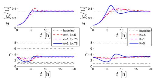
**Figure 6.7:** Effect of  $\mu$  estimation error on controller performance using the proposed (left) and (6.25) (right) controllers. Initial condition:  $(x_0, s_0, \gamma_0) = (.05, .01, 3)$ , set-point:  $(x^*, s^*, \gamma^*) = (1/3, 2.86, 3)$ .
