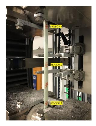
Figure 6. Sensorized beam test piece setting.
