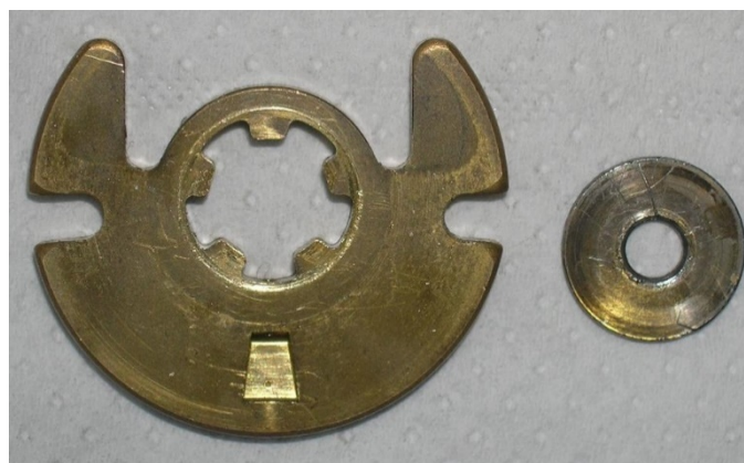
FIG 23: DAMAGED THRUST BEARING AFTER QUASI-ADIABATIC TESTS
