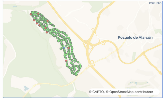
FIGURE 2. Water meters in the geographical area. A K-means clustering is performed to group the water meters into 3 groups: High, medium and low consumption groups.
