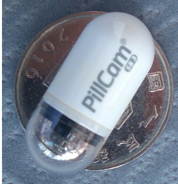
Figure 2.1: The PillCam SB 3, which is the capsule endoscope model used in this work.
