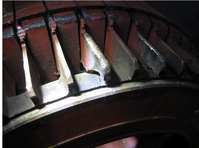
**Figure 7.1:** Motor of Appendix 7.7 (3.15 MW), with a broken bar fault.
