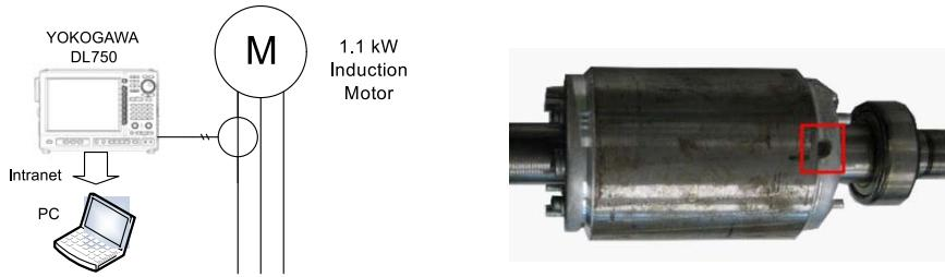
**Figure 6.10:** Experimental setup: measurement equipment (left), and rotor of the motor whose characteristics are given in Appendix 6.9, with a broken bar (right).
