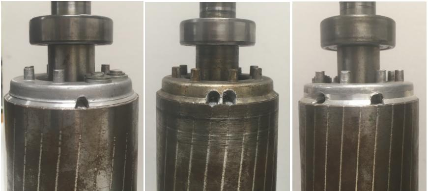
**Figure 6.11:** Tested rotors with faulty cages: one broken bar (left), two consecutive broken bars (centre) and two non-consecutive broken bars (right).
