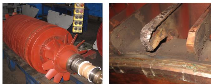
**Figure 7.6:** Rotor of the tested 3.15 MW IM (left), and close-up view of the broken bar (right).
