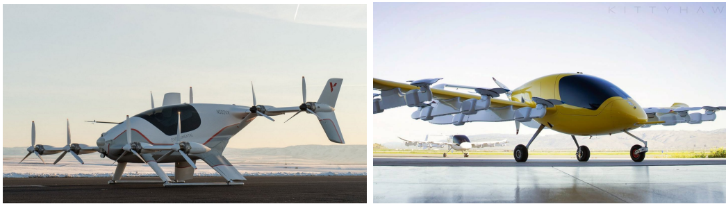
Figure 2.2: Current advanced prototypes for air taxis in the form of eVTOL by Airbus (left) and Zephyr Airworks (right).
