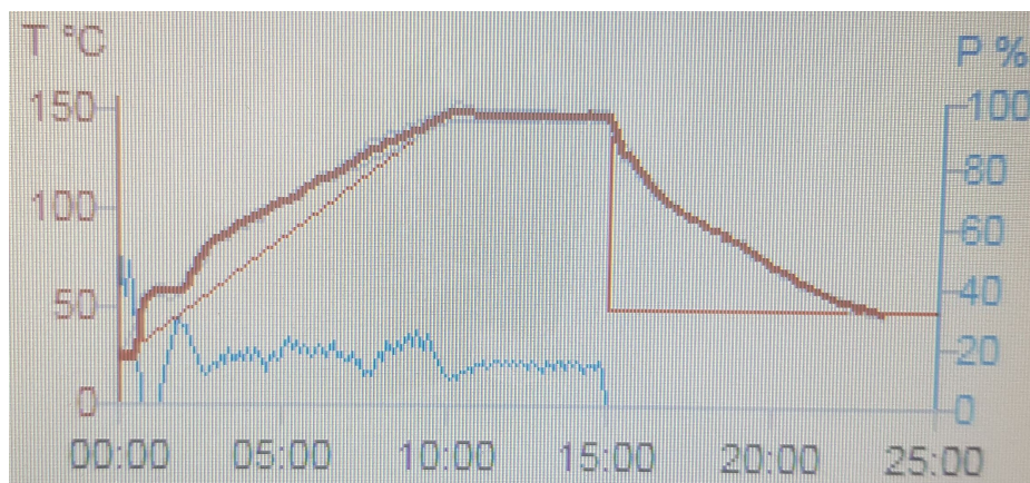
Figure 40: Graph of the temperature evolution and the power (p) during the digestion as a function of time for the HF process
