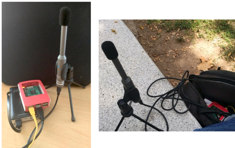
Fig. 5. On the left side: Acoustic node formed by a Raspberry Pi encapsulated in a protective case and connected to a battery (below) and a microphone. On the right side: The acoustic node placed at one of the sites described in Section 3.
