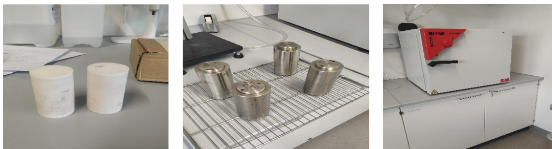
Figure 3: A) Teflon liners, B) autoclaves used for the synthesis. C) Oven used for hydrothermal process
